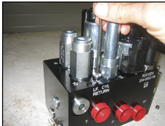
FIGURE 5. Port Plug Reinstalled on the AutoBoom Valve
