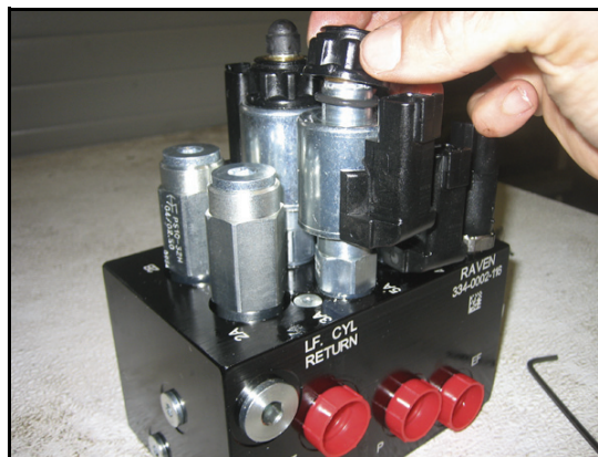
FIGURE 6. Coil Reinstalled on the AutoBoom Valve
