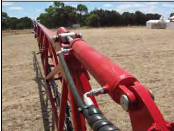
FIGURE 10. Cylinder Hoses Installed
