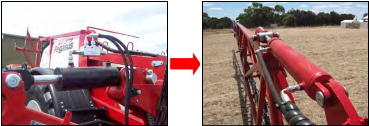
FIGURE 4. New Tilt Cylinders Installed
