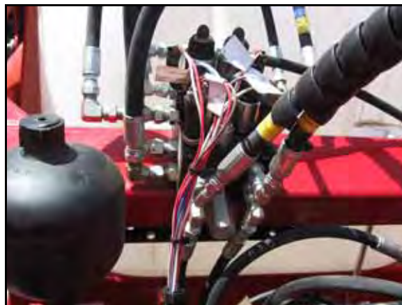
FIGURE 5. Cylinder Hoses Installed on the AutoBoom Valve
