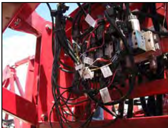
FIGURE 3. Machine's Center Boom Function Coils
