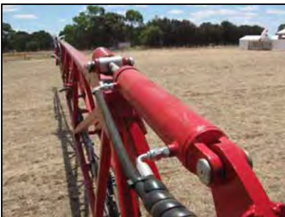
FIGURE 8. Cylinder Hoses Installed
