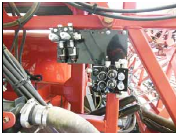
FIGURE 18. Valve Mounting Bracket Installed on the Machine
