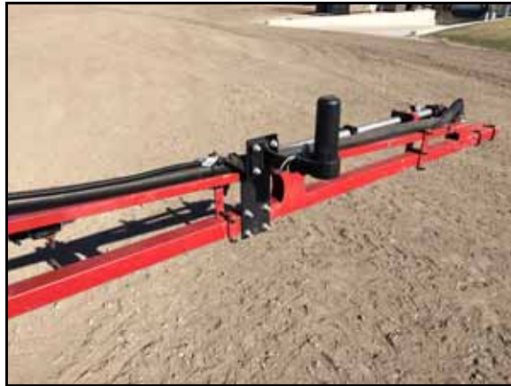
FIGURE 4. Left Outer Boom Sensor Installed
