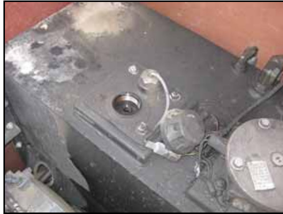
FIGURE 29. Oil Reservoir Cap Removed
