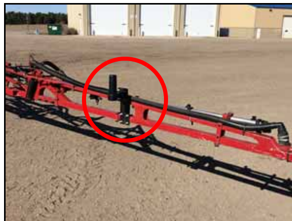
FIGURE 9. Outer Sensor Installation Location
