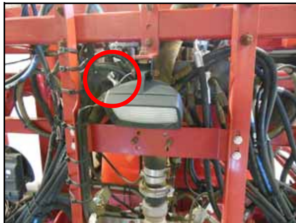
FIGURE 38. Machine's Left Down Hose
