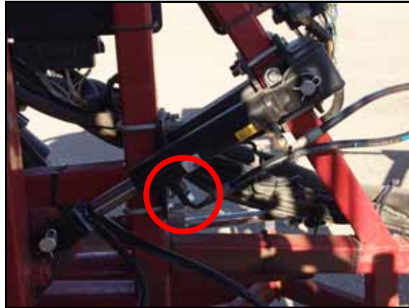
FIGURE 46. Rod-End Left UltraGlide XT Cylinder Hose Installed
