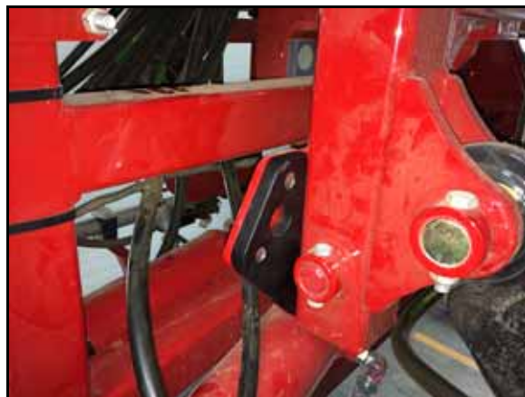
FIGURE 7. Lower Cylinder Support Bracket Installed
