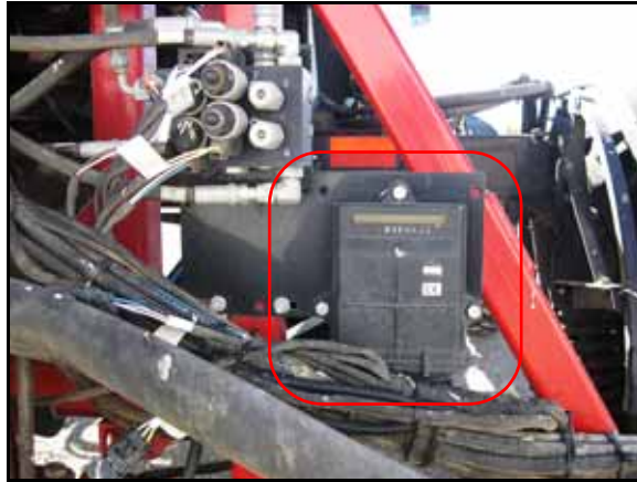
FIGURE 19. Existing AutoBoom Node to be Removed
