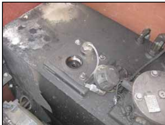
FIGURE 22. Oil Reservoir Cap Removed
