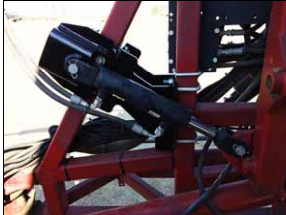
FIGURE 15. Hydraulic Cylinders Installed
