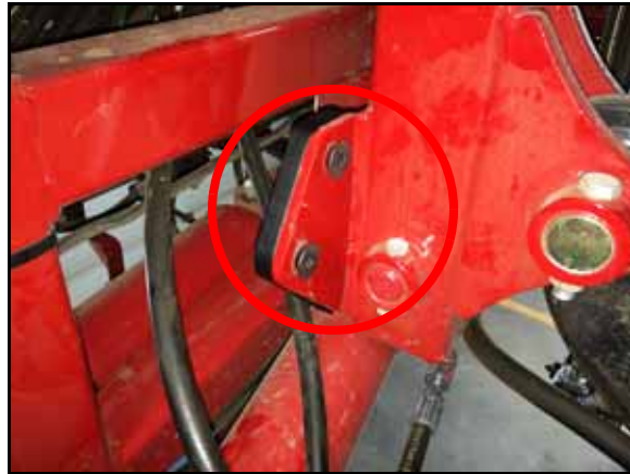
FIGURE 5. Lower Cylinder Support Bracket Secured to Shock Mounting Tab
