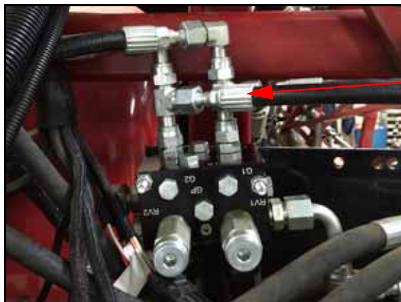
FIGURE 45. Base-End Right Cylinder Hose Installed on UltraGlide XT Valve
