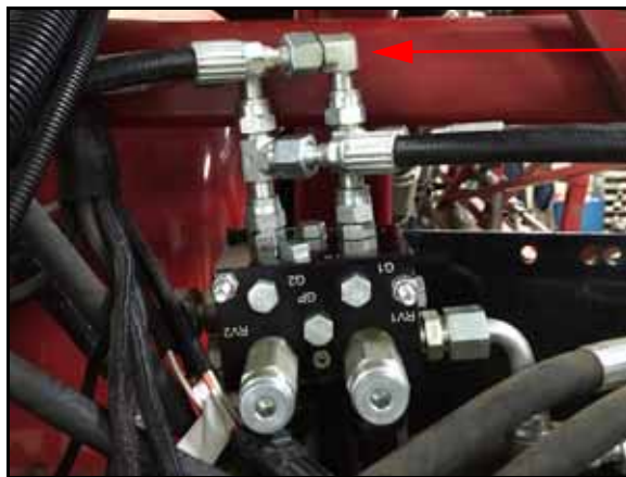
FIGURE 49. Base-End Left Cylinder Hose Installed on UltraGlide XT Valve
