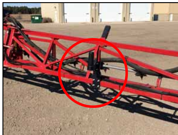
FIGURE 10. Left Inner Sensor Installed
