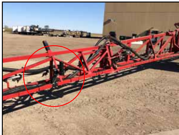
FIGURE 6. Right Inner Boom Sensor Installed
