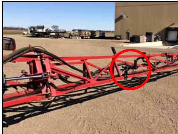
FIGURE 3. Left Inner Boom Sensor Installed
