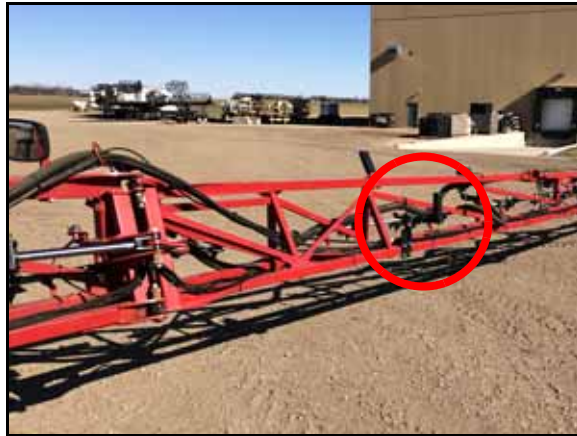
FIGURE 4. Left Inner Boom Sensor Installed
