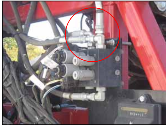
FIGURE 3. Pressure and Tank Hoses Installed
