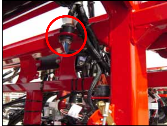
FIGURE 3. AutoBoom Harness Cable Installed
