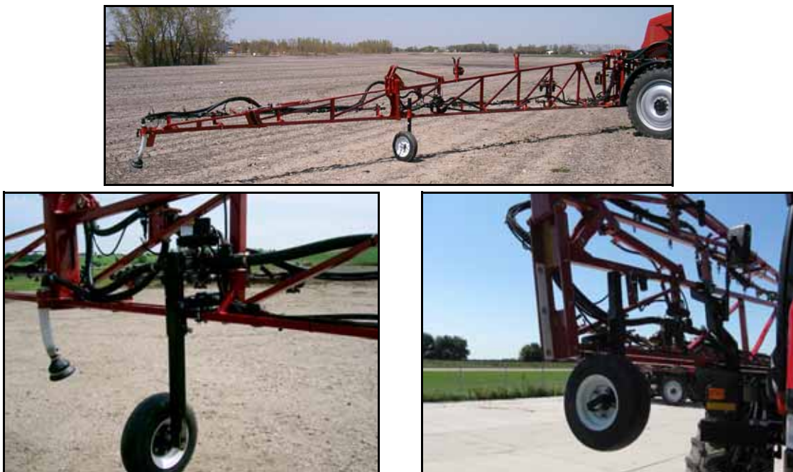
FIGURE 1. Gauge Wheel Installed
