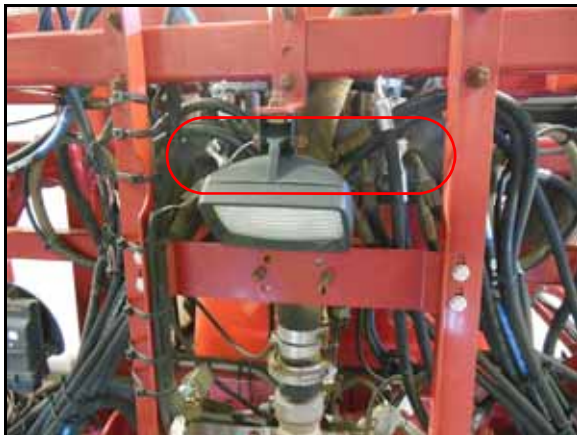
FIGURE 5. Left and Right Down Hoses Installed
