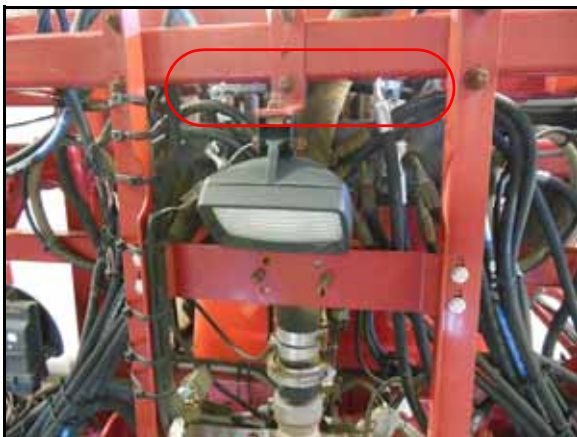
FIGURE 4. Left and Right Cylinder Hoses Installed
