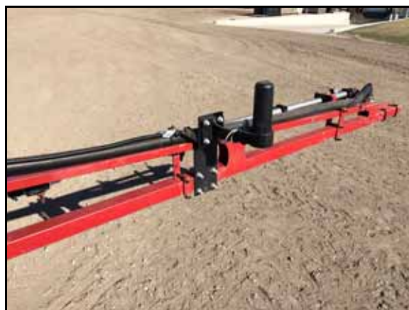
FIGURE 3. Left Boom Sensor Installed
