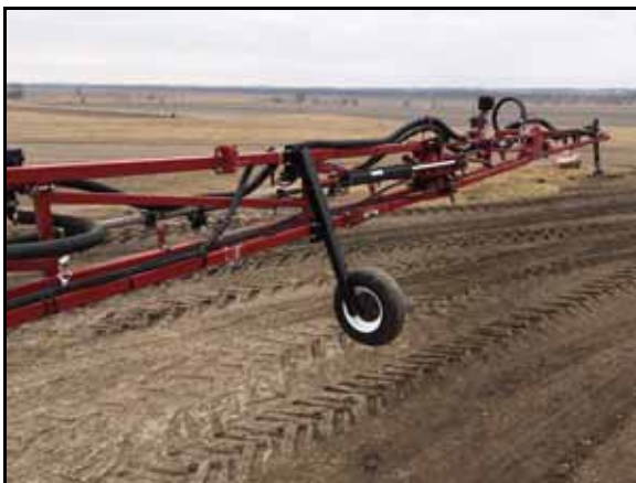
FIGURE 2. Gauge Wheel Installed
