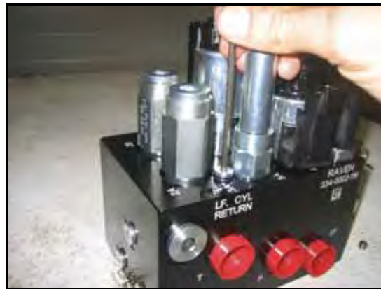
FIGURE 5. Port Plug Reinstalled on the AutoBoom Valve
