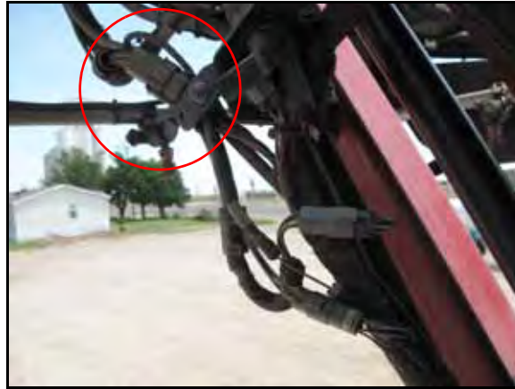
FIGURE 14. Machine's CAN and Power Connection
