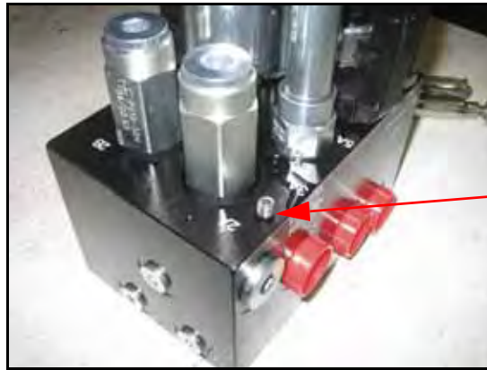
FIGURE 4. Orifice Fitting Removed from the AutoBoom Valve
