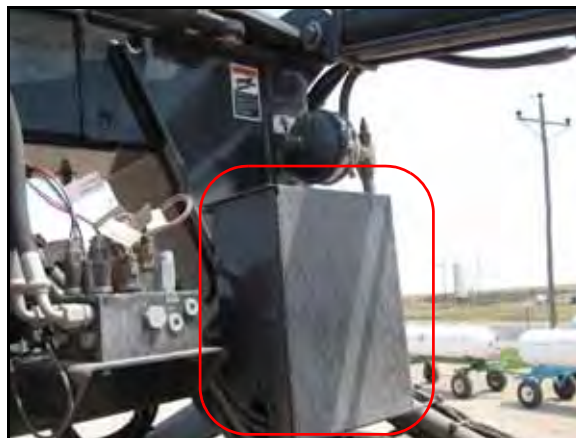
FIGURE 9. AutoBoom Node Mounting Location
