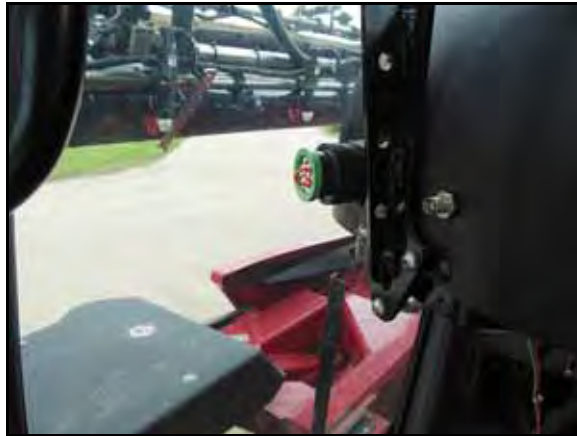
FIGURE 13. Node Power Jumper Installed
