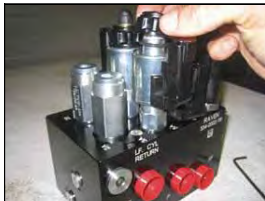
FIGURE 6. Coil Reinstalled on the AutoBoom Valve
