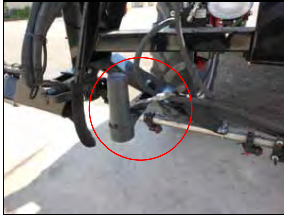
FIGURE 7. Center Rack Sensor Mounting
