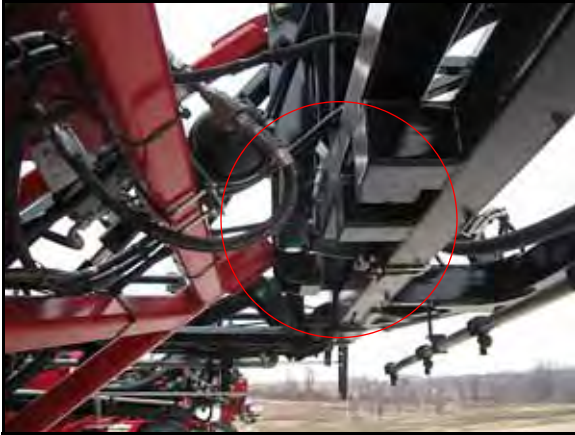
FIGURE 9. Center Sensor Mounting Location
