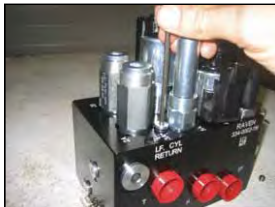
FIGURE 5. Port Plug Reinstalled on the AutoBoom Valve
