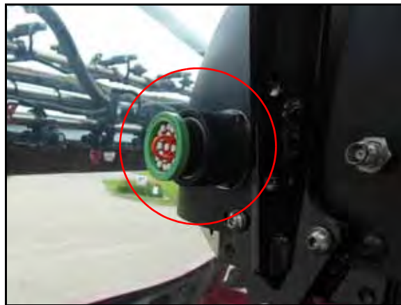
FIGURE 14. Node Power Jumper Installed
