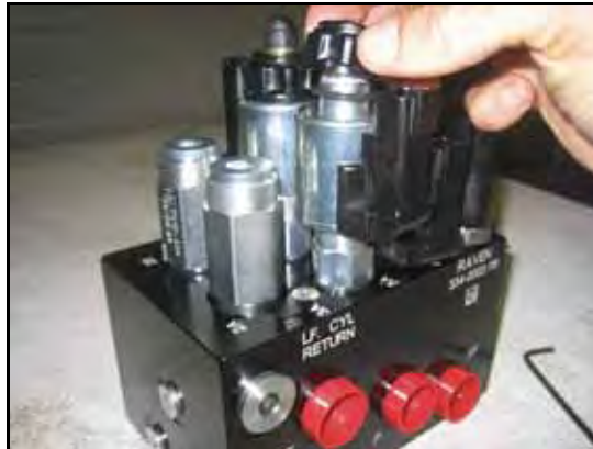
FIGURE 6. Coil Reinstalled on the AutoBoom Valve
