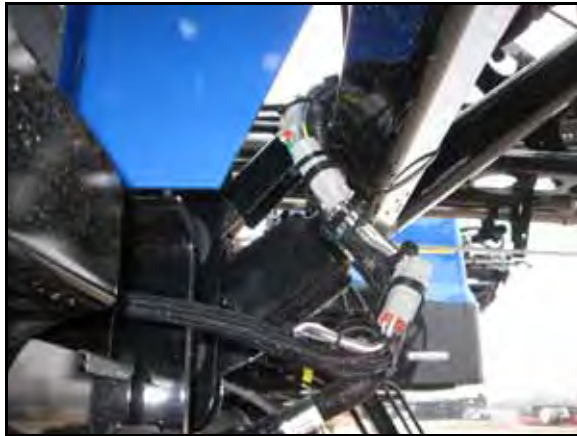
FIGURE 12. AutoBoom Harness Connected to the Machine's Harness
