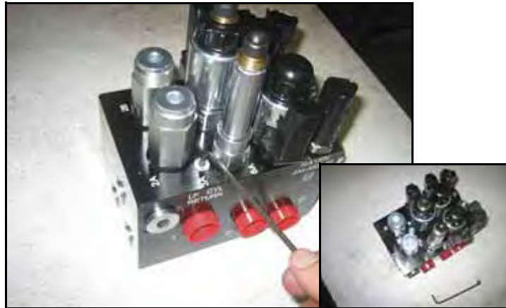
FIGURE 3. Port Plugs Removed from the AutoBoom Valve
