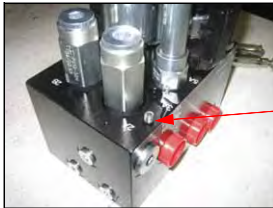
FIGURE 4. Orifice Fitting Removed from the AutoBoom Valve
