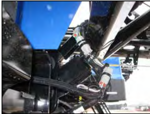
FIGURE 12. AutoBoom Harness Connected to the Machine's Harness
