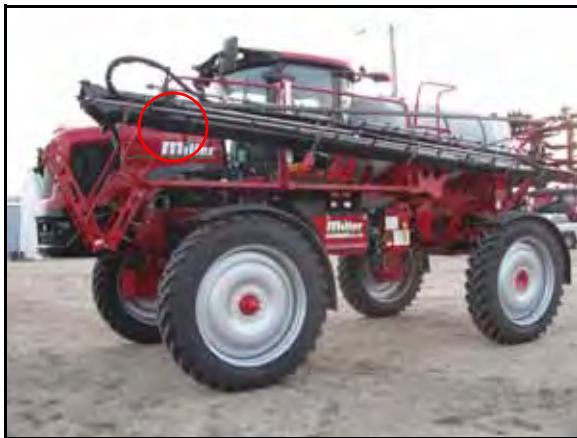
FIGURE 11. Gauge Wheel Mounting Location
