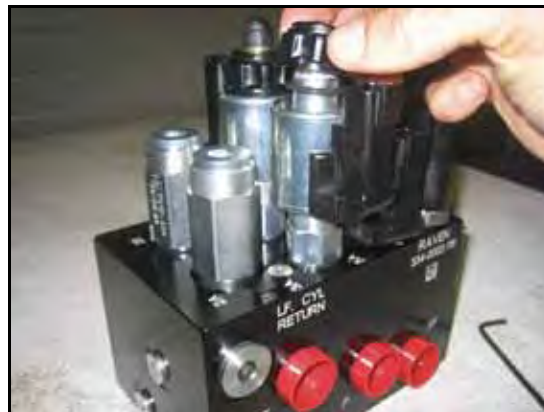
FIGURE 6. Coil Reinstalled on the AutoBoom Valve
