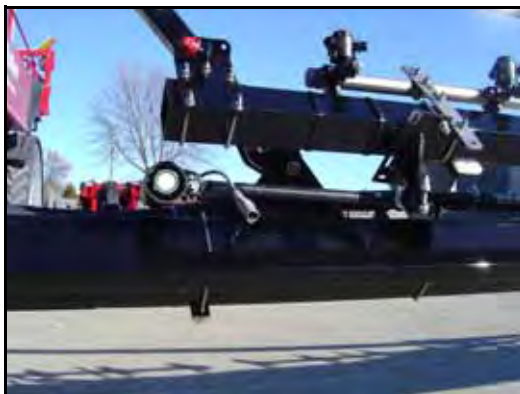
FIGURE 8. Installed Boom Sensors
