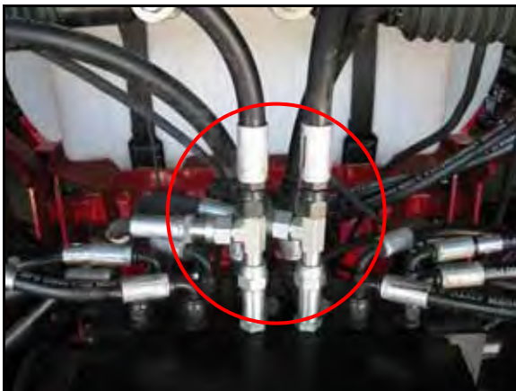
FIGURE 10. Left and Right Cylinder Hoses Installed
