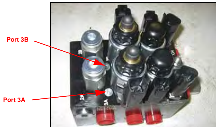
FIGURE 1. Port 3A and 3B Location
