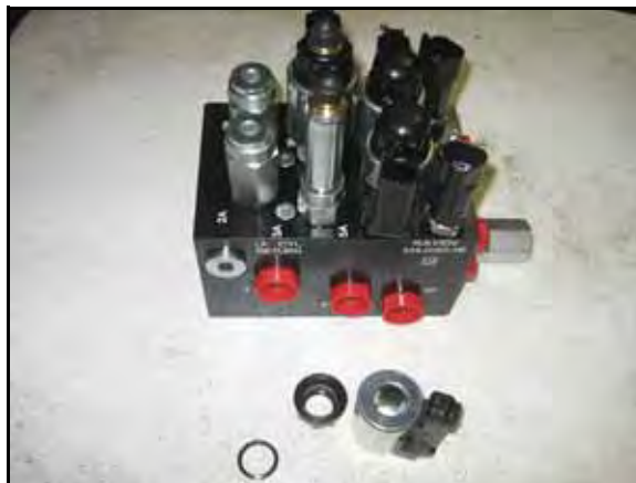
FIGURE 2. Coil Removed from the AutoBoom Valve
