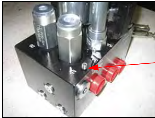
FIGURE 4. Orifice Fitting Removed from the AutoBoom Valve
