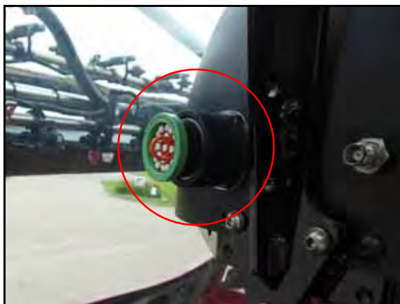
FIGURE 14. Node Power Jumper Installed
