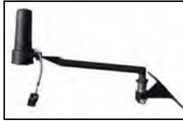
FIGURE 7. Sensor Installed on Mounting Bracket
