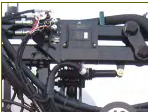
FIGURE 11. AutoBoom Node Mounting Location
