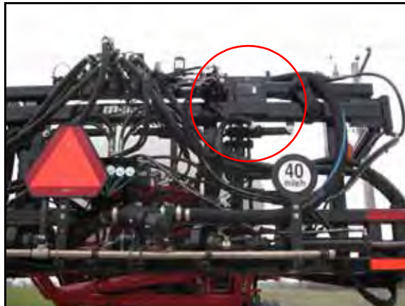
FIGURE 8. AutoBoom Valve Mounted on the Sprayer
