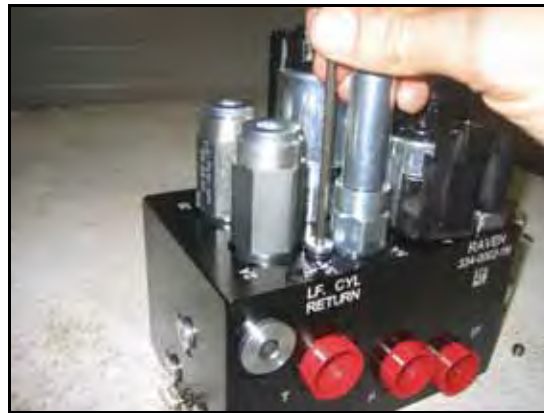
FIGURE 5. Port Plug Reinstalled on the AutoBoom Valve
