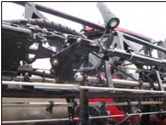
FIGURE 9. Center Rack Sensor Mounting
