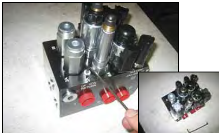
FIGURE 3. Port Plugs Removed from the AutoBoom Valve
