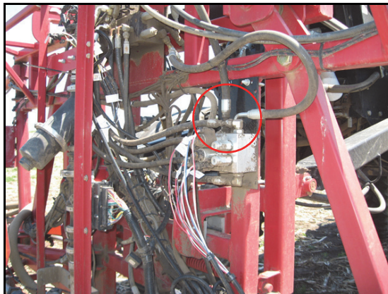
FIGURE 9. Pressure and Tank Hoses Installed
