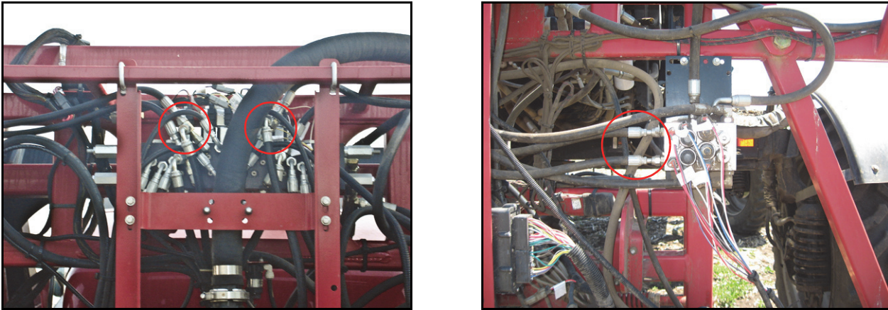
FIGURE 10. Left and Right Cylinder Hoses Installed
