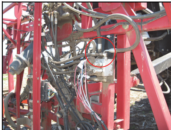
FIGURE 3. Pressure and Tank Hoses Installed
