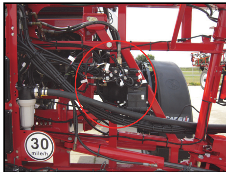
FIGURE 2. AutoBoom Valve Mounted on the Machine
