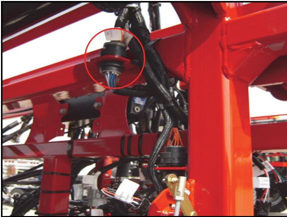
FIGURE 12. AutoBoom Harness Cable Installed
