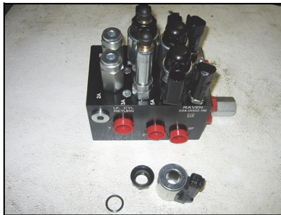
FIGURE 2. Coil Removed from the AutoBoom Valve
