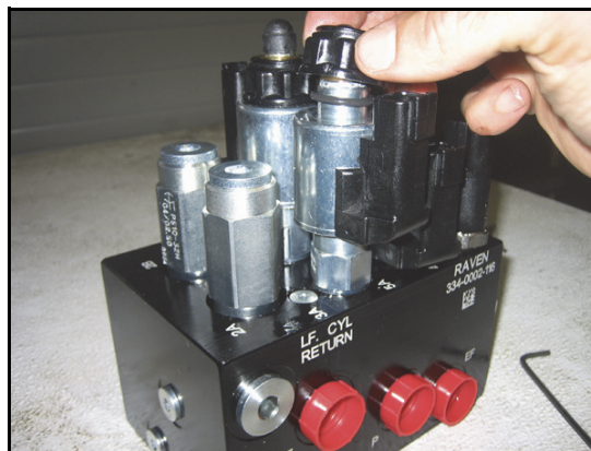
FIGURE 6. Coil Reinstalled on the AutoBoom Valve
