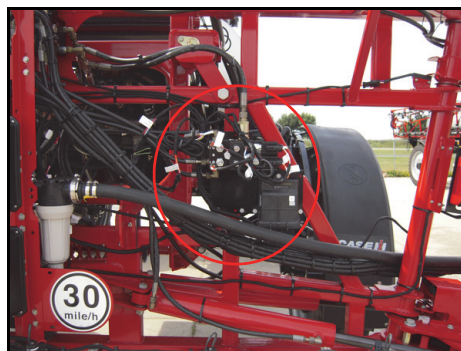
FIGURE 8. AutoBoom Valve Mounted on the Machine
