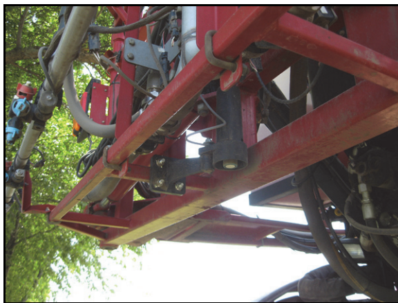
FIGURE 9. Mounted Center Rack Sensor
