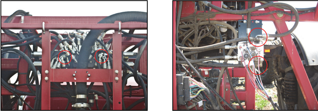
FIGURE 5. Left and Right Down Hoses Installed
