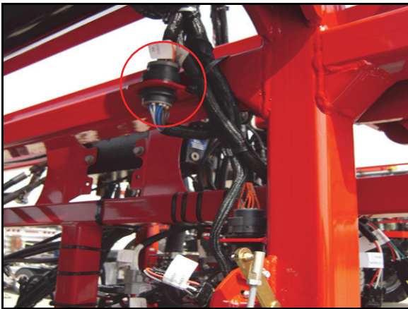
FIGURE 14. AutoBoom Harness Cable Installed
