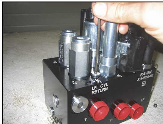
FIGURE 5. Port Plug Reinstalled on the AutoBoom Valve
