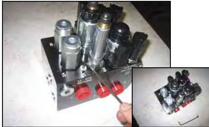
FIGURE 3. Port Plugs Removed from the AutoBoom Valve
