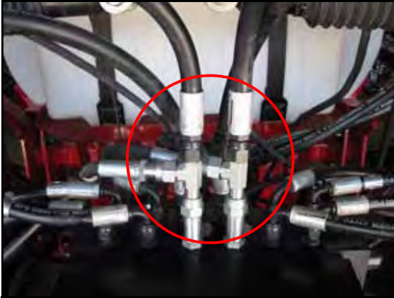
FIGURE 10. Left and Right Cylinder Hoses Installed
