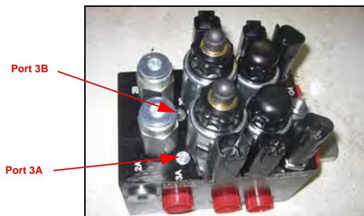
FIGURE 1. Port 3A and 3B Location
