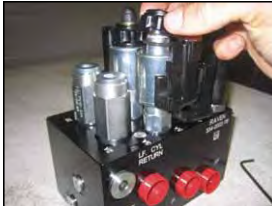
FIGURE 6. Coil Reinstalled on the AutoBoom Valve
