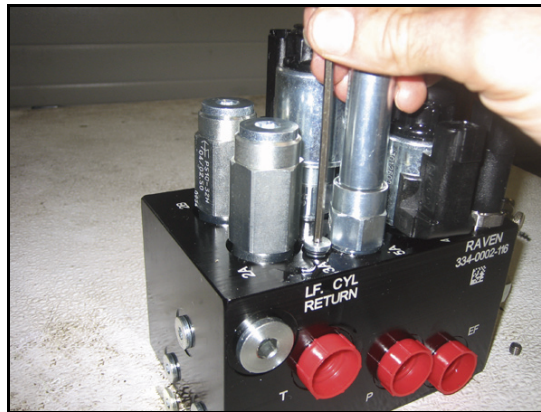
FIGURE 5. Port Plug Reinstalled on the AutoBoom Valve
