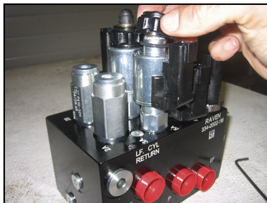
FIGURE 6. Coil Reinstalled on the AutoBoom Valve
