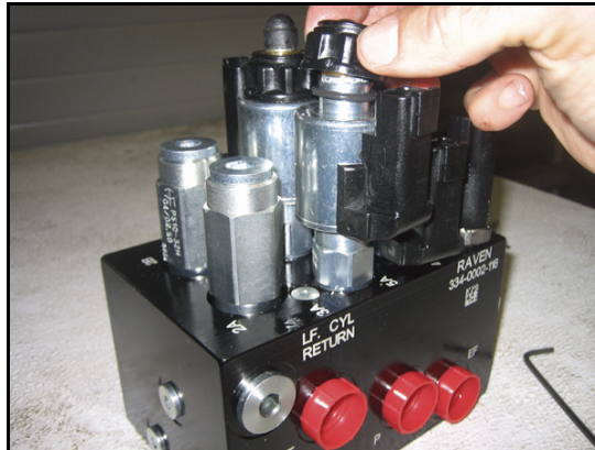
FIGURE 6. Coil Reinstalled on the AutoBoom Valve
