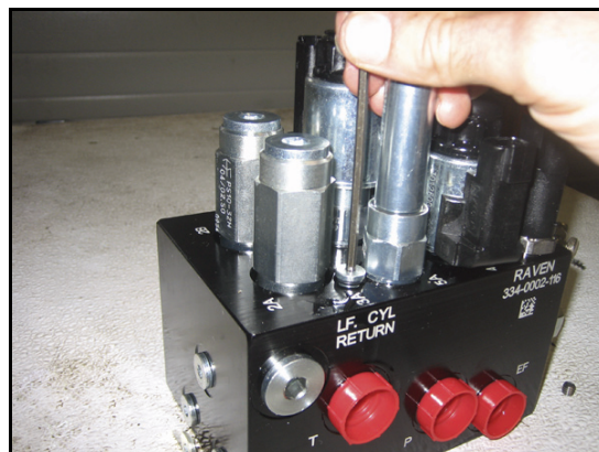
FIGURE 5. Port Plug Reinstalled on the AutoBoom Valve
