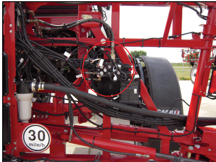
FIGURE 2. AutoBoom Valve Mounted on the Sprayer
