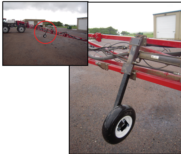
FIGURE 12. Gauge Wheel Installed
