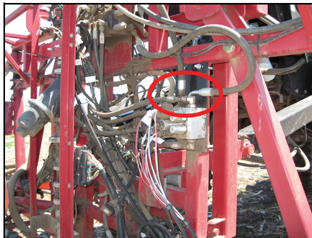
FIGURE 9. Pressure and Tank Hoses Installed
