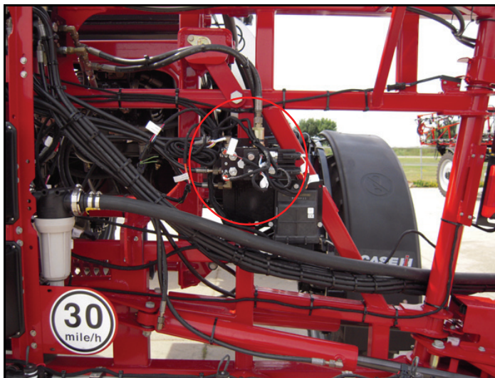
FIGURE 8. AutoBoom Valve Mounted on the Sprayer
