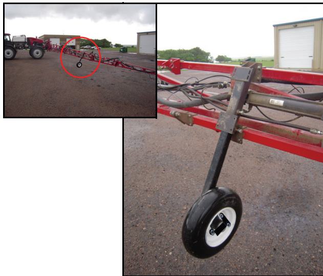
FIGURE 8. Gauge Wheel Installed
