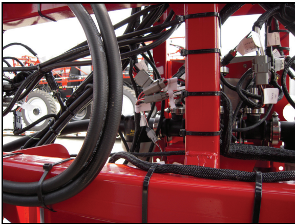
FIGURE 10. AutoBoom Harness Cable Installed
