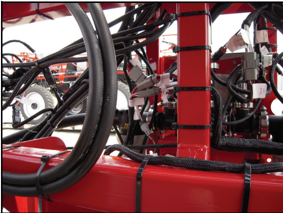
FIGURE 14. AutoBoom Harness Cable Installed
