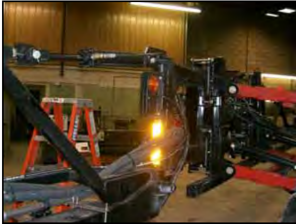
FIGURE 11. Cylinder Hoses Installed
