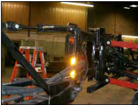
FIGURE 5. Cylinder Hoses Installed
