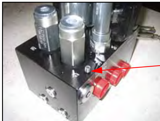
FIGURE 5. Orifice Fitting Removed from the AutoBoom Valve
