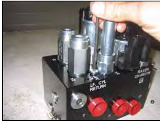
FIGURE 6. Port Plug Reinstalled on the AutoBoom Valve
