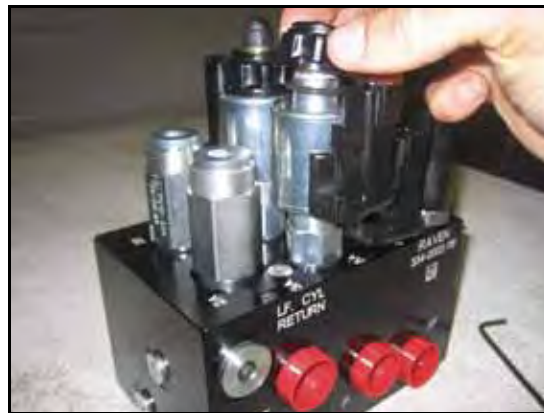
FIGURE 7. Coil Reinstalled on the AutoBoom Valve
