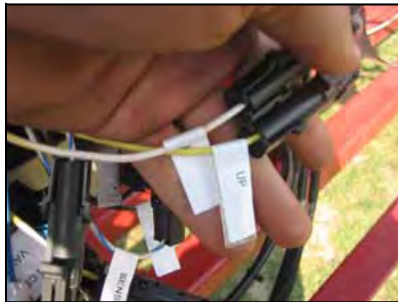
FIGURE 7. Machine's Up Cylinder Wiring
