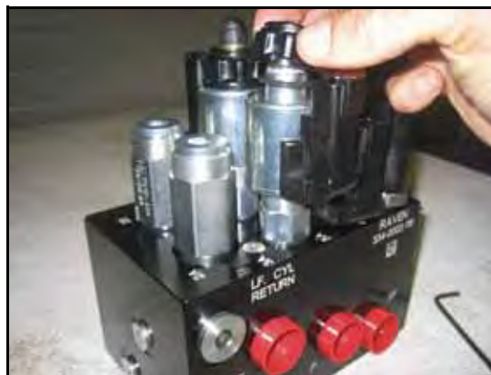
FIGURE 6. Coil Reinstalled on the AutoBoom Valve
