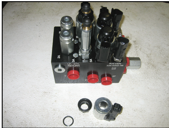
FIGURE 3. Coil Removed from the AutoBoom Valve
