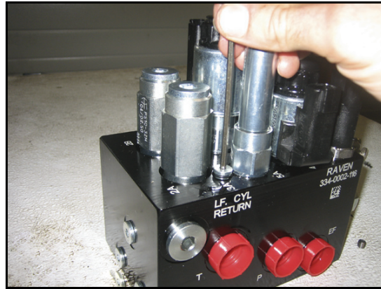
FIGURE 6. Port Plug Reinstalled on the AutoBoom Valve
