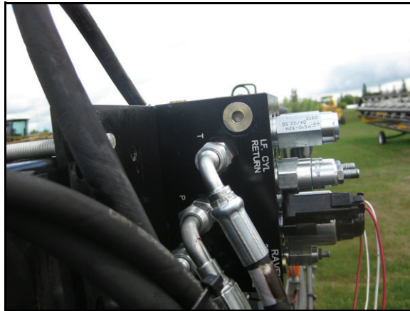
FIGURE 5. Pressure and Tank Lines Installed
