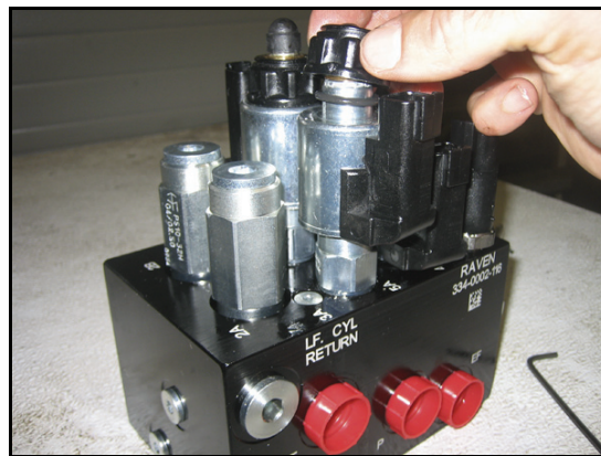
FIGURE 7. Coil Reinstalled on the AutoBoom Valve
