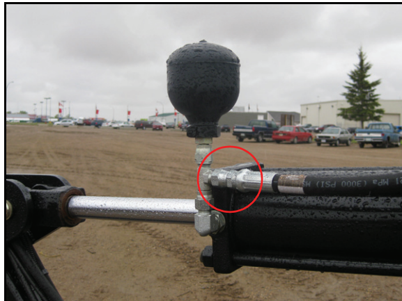
FIGURE 7. Hydraulic Hoses Installed on Machine's Cylinders
