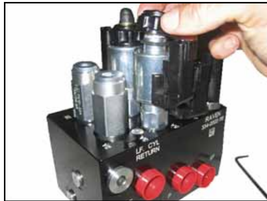
FIGURE 7. Coil Reinstalled on the AutoBoom Valve
