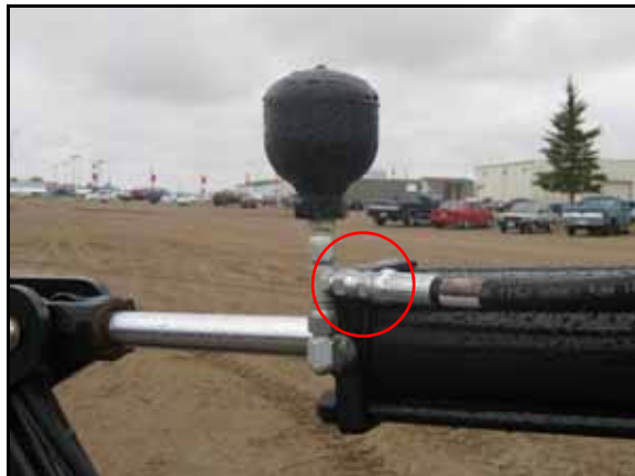
FIGURE 13. Hydraulic Hoses Installed on Machine's Cylinders
