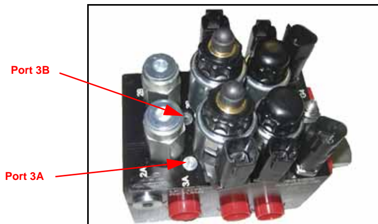
FIGURE 2. Port 3A and 3B Location
