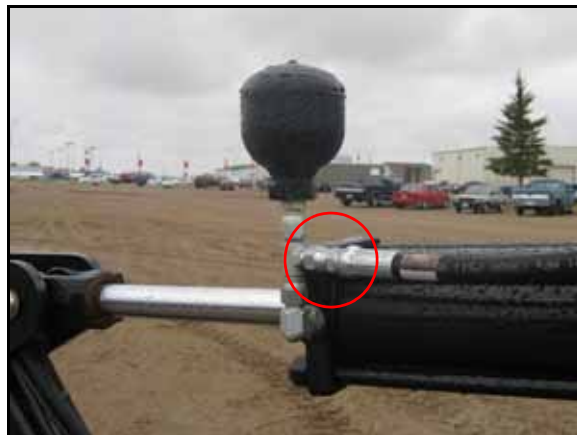
FIGURE 7. Hydraulic Hoses Installed on Machine's Cylinders
