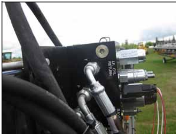
FIGURE 5. Pressure and Tank Lines Installed
