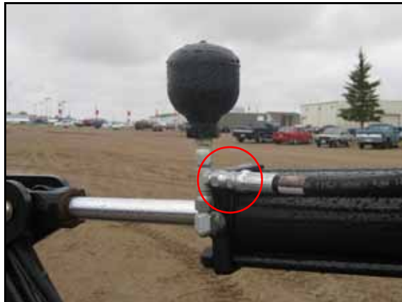
FIGURE 7. Hydraulic Hoses Installed on Machine's Cylinders
