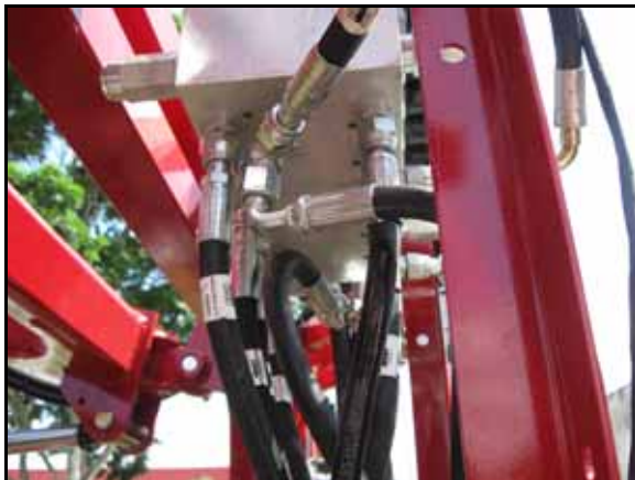
FIGURE 6. Left Down Hose Installed
