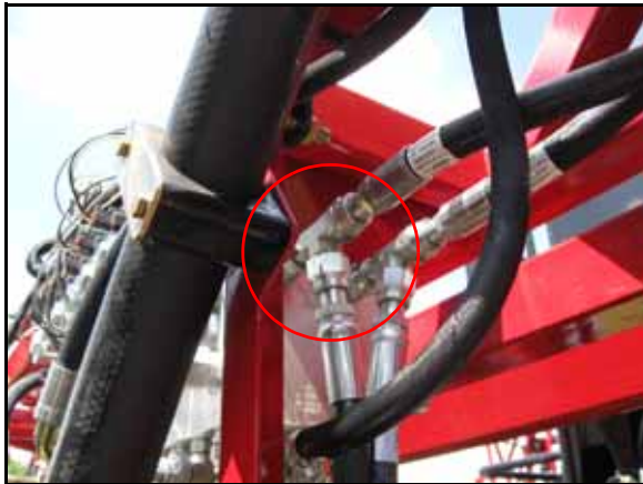
FIGURE 2. Pressure Hose Installed
