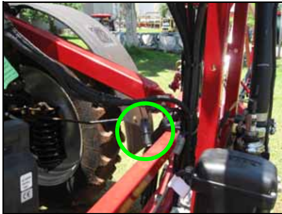
FIGURE 9. Machine's Existing Power Connection
