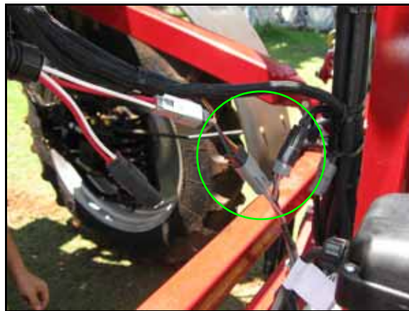
FIGURE 6. AutoBoom Harness Installed on Machine's CAN Connections
