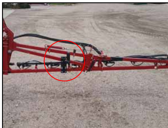
FIGURE 3. Left Boom Sensor Installed
