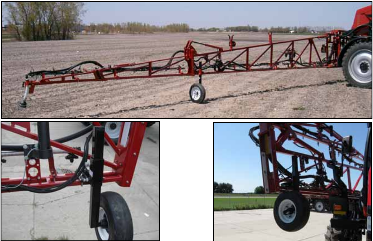
FIGURE 1. Gauge Wheel Installed
