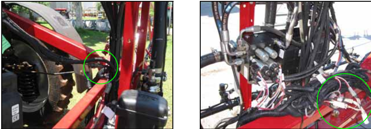
FIGURE 5. Machine's Existing CAN Connection
