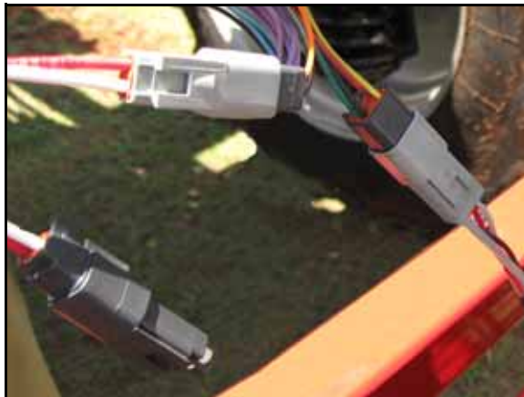
FIGURE 10. AutoBoom Harness Cable Power Connection
