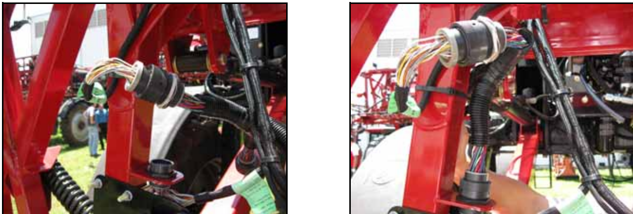
FIGURE 4. AutoBoom Harness Connected to Machine's Harness Connections
