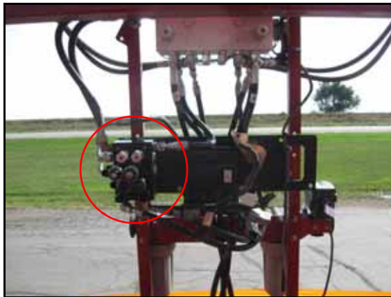
FIGURE 1. AutoBoom Valve Mounted on the Machine
