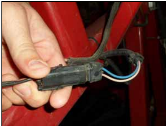
FIGURE 8. Extension Cable Connected to AutoBoom Harness
