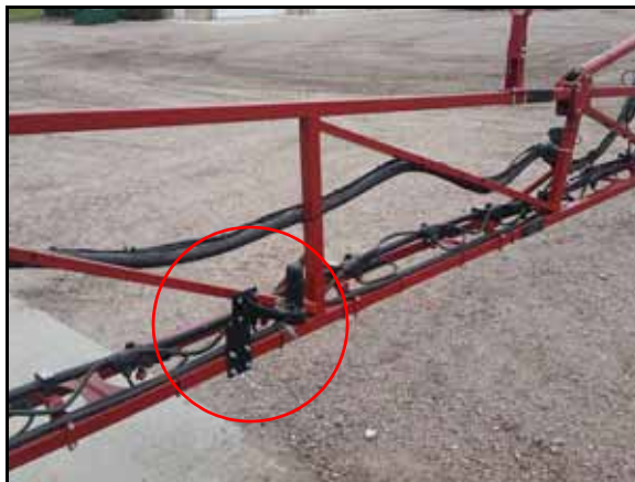
FIGURE 4. Left Inner Boom Sensor Installed
