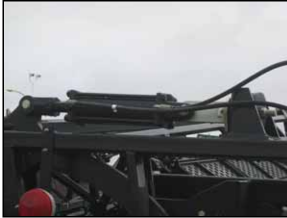
FIGURE 7. Hydraulic Hoses Installed on Machine's Cylinders
