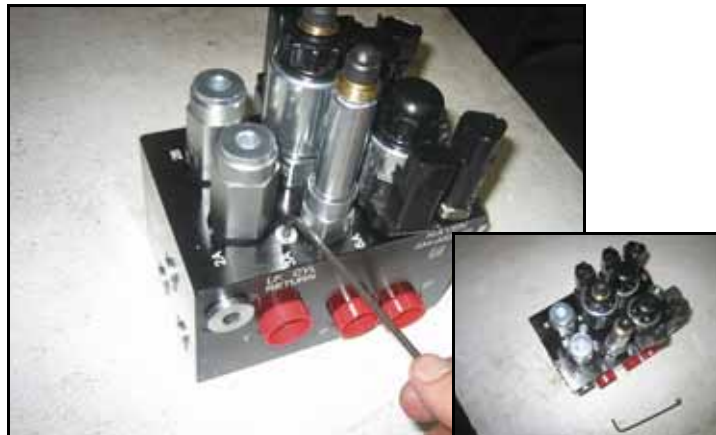
FIGURE 4. Port Plugs Removed from the AutoBoom Valve
