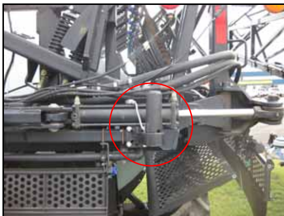
FIGURE 11. Center Sensor Mounting Location
