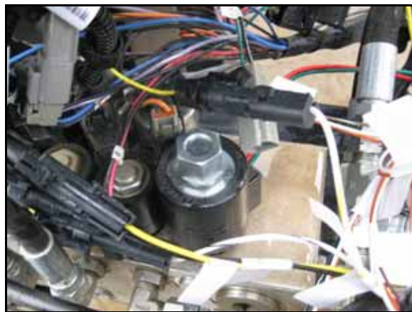
FIGURE 16. Open Center Dump Valve Coil
