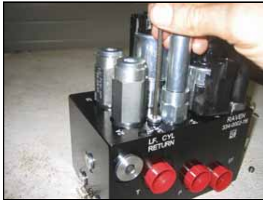
FIGURE 6. Port Plug Reinstalled on the AutoBoom Valve
