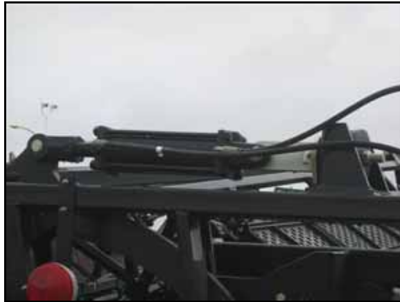
FIGURE 7. Hydraulic Hoses Installed on Machine's Cylinders
