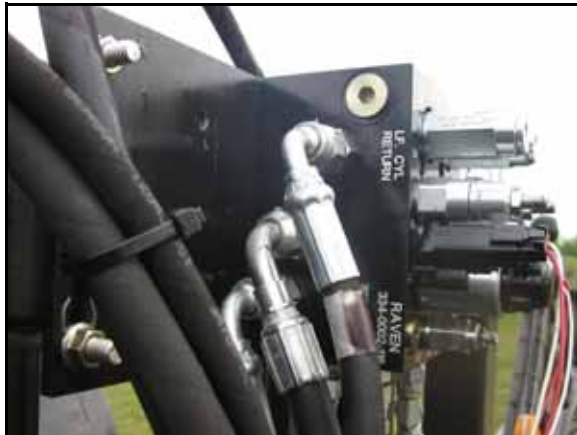
FIGURE 5. Pressure and Tank Lines Installed
