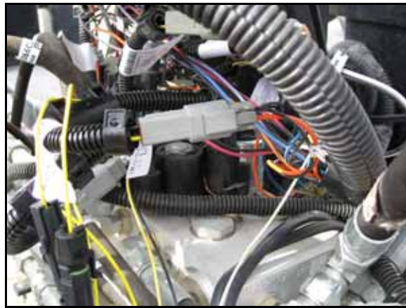
FIGURE 15. Machine's Center Boom Function Coils
