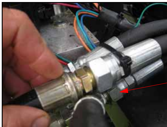
FIGURE 10. Extension Hose Installed on Machine's Pressure Hose
