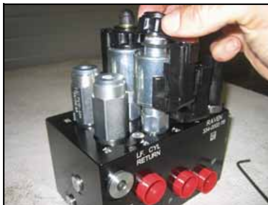
FIGURE 7. Coil Reinstalled on the AutoBoom Valve
