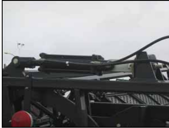
FIGURE 13. Hydraulic Hoses Installed on Machine's Cylinders
