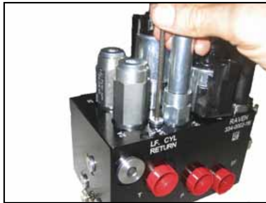
FIGURE 5. Port Plug Reinstalled on the AutoBoom Valve
