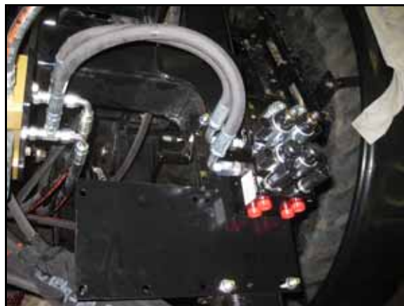
FIGURE 8. AutoBoom Valve Mounted on the Sprayer
