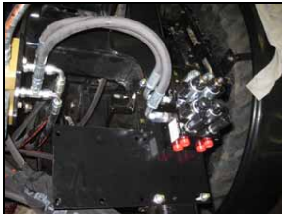
FIGURE 2. AutoBoom Valve Mounted on the Sprayer
