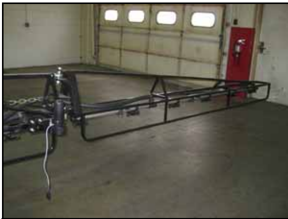
Outer Boom Sensor Mounting Location
