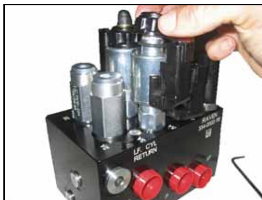
FIGURE 6. Coil Reinstalled on the AutoBoom Valve
