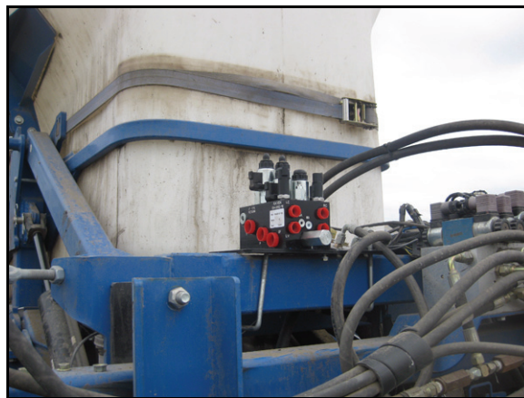
FIGURE 3. AutoBoom Valve Mounting on the Machine
