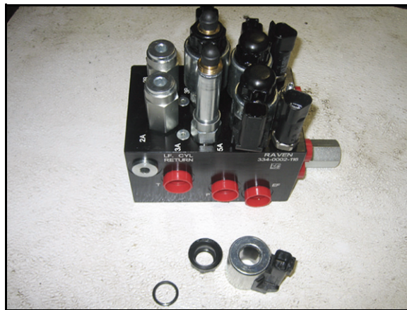
FIGURE 2. Coil Removed from the AutoBoom Valve
