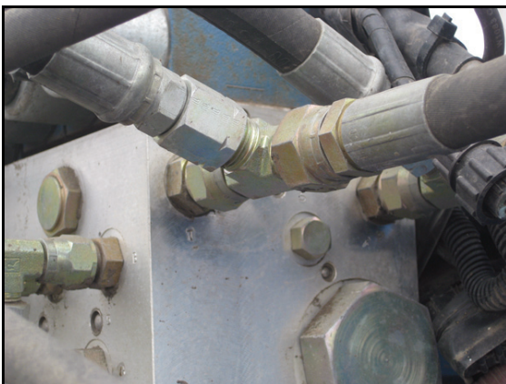
FIGURE 5. Tank Hose Installed
