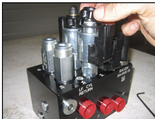
FIGURE 6. Coil Reinstalled on the AutoBoom Valve
