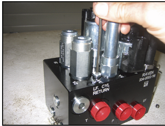
FIGURE 5. Port Plug Reinstalled on the AutoBoom Valve
