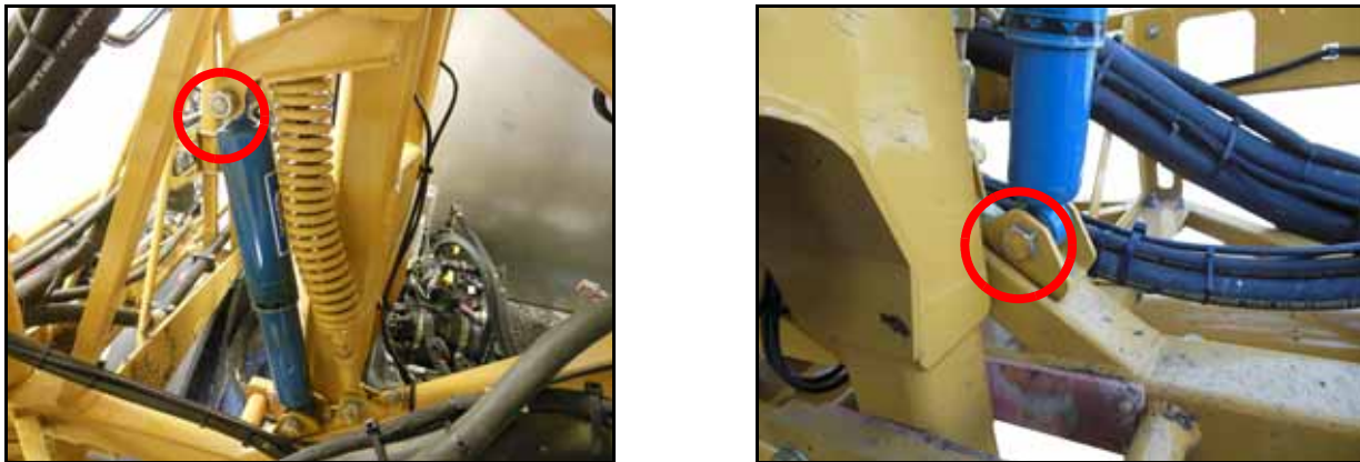
FIGURE 14. Shock Absorber Bolt to be Removed - 120' Booms
