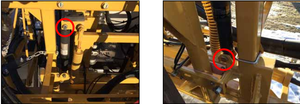
FIGURE 14. Shock Absorber Bolt to be Removed - 120' Booms
