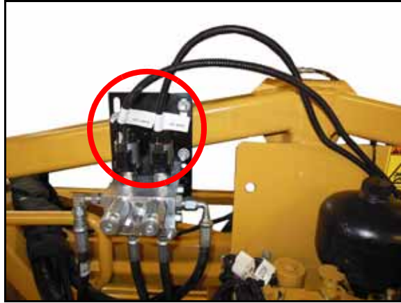
FIGURE 28. Slant Connectors Installed
