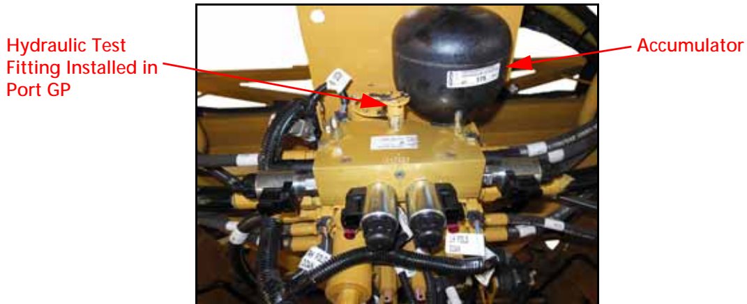
FIGURE 3. AutoBoom Valve Mounted to the Machine's Hydraulic Valve
