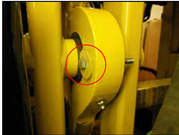
FIGURE 9. Pivot Bearing Bolt to be Removed
