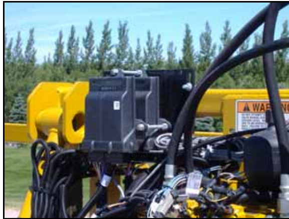
FIGURE 22. Installed AutoBoom Node
