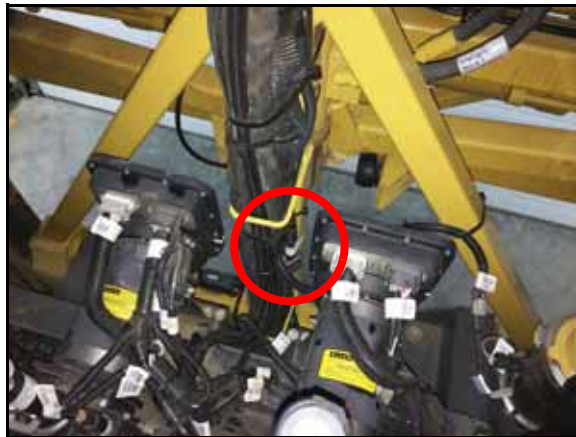
FIGURE 29. 12-Pin Connector Connected to AGCO Harness
