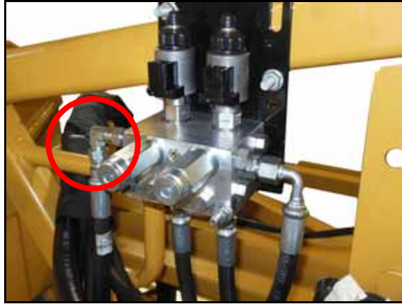
FIGURE 11. Tank Hose Installed on UltraGlide XT Valve
