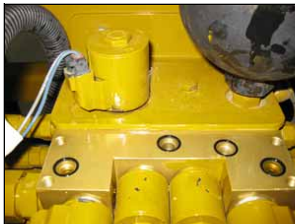
FIGURE 2. O-Rings Installed on the Machine's Hydraulic Valve
