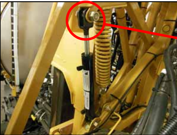
FIGURE 16. Cylinder Installed - 120' Booms
