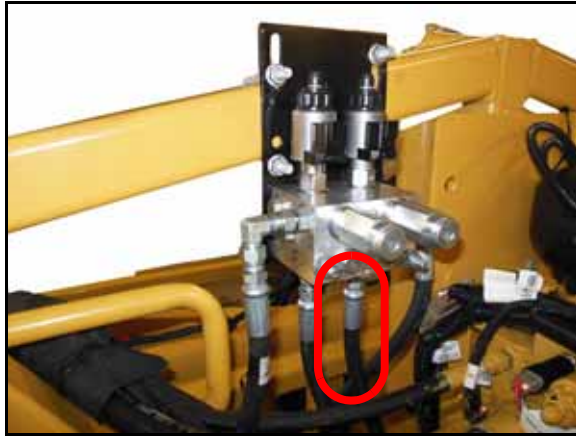
FIGURE 20. Hose Installed on UltraGlide XT Valve
