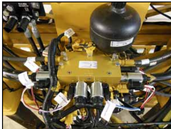
FIGURE 5. Valve Harness Installed on the AutoBoom Valve
