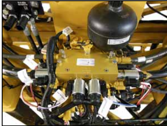
FIGURE 19. Valve Harness Installed on the AutoBoom Valve
