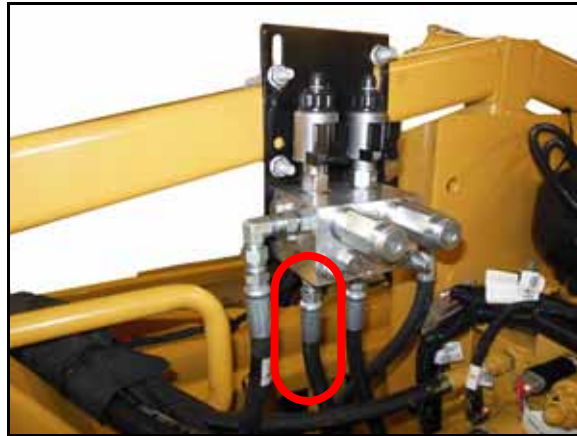
FIGURE 17. Hose Installed on UltraGlide XT Valve
