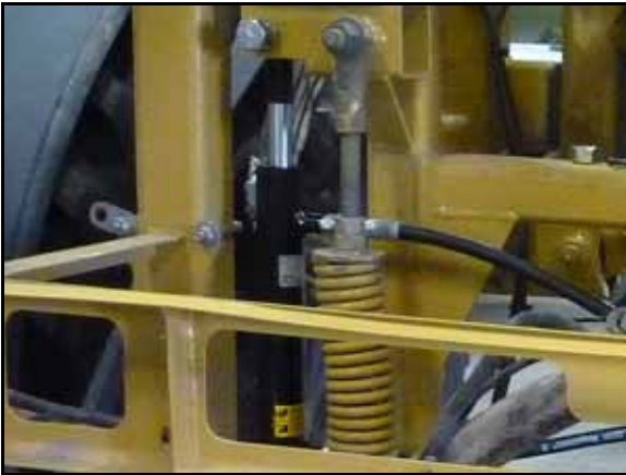
FIGURE 16. Cylinder Installed - 120' Booms
