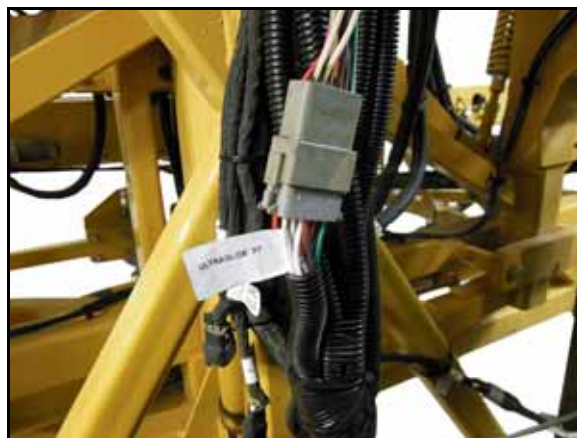
FIGURE 27. Valve Harness Connected to Auxiliary Sensor Cable
