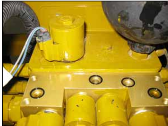
FIGURE 2. O-Rings Installed on the Machine's Hydraulic Valve
