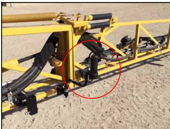
FIGURE 5. Mounted Boom Sensor
