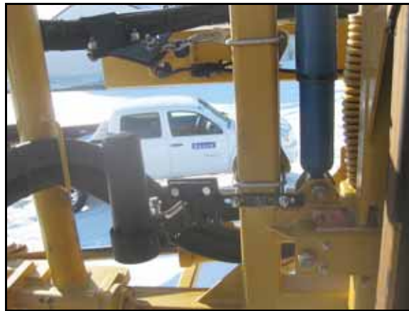
FIGURE 6. Center Rack Sensor Installed
