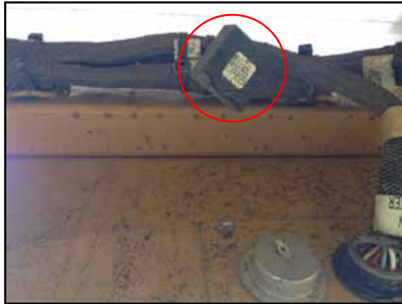
FIGURE 16. Machine's Existing CAN Terminator
