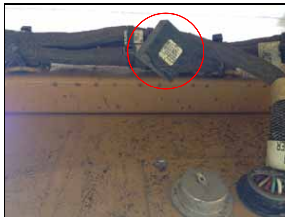
FIGURE 12. Machine's Existing CAN Terminator
