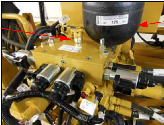
FIGURE 3. AutoBoom Valve Mounted to the Machine's Hydraulic Valve
