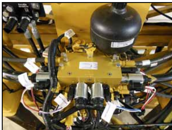
FIGURE 11. Valve Harness Installed on the AutoBoom Valve
