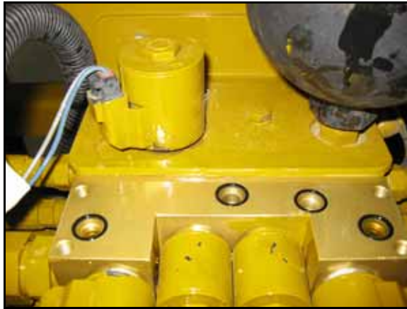
FIGURE 2. O-Rings Installed on the Machine's Hydraulic Valve
