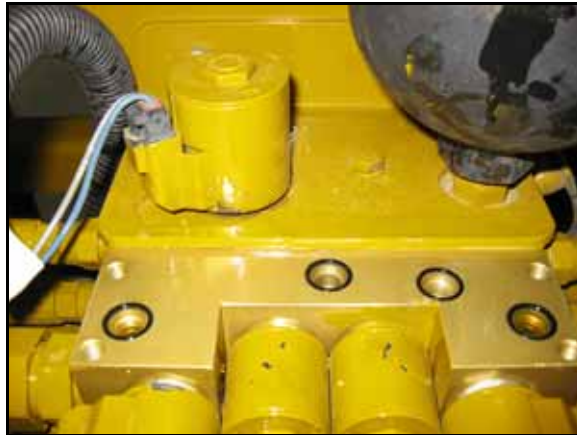
FIGURE 2. O-Rings Installed on the Machine's Hydraulic Valve
