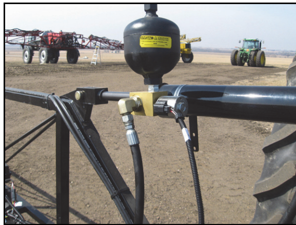
FIGURE 11. Left and Right Cylinder Hoses Installed
