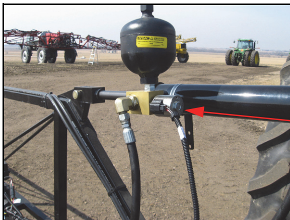
FIGURE 5. Left and Right Cylinder Hoses Installed
