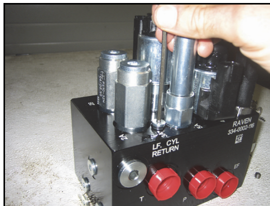
FIGURE 5. Port Plug Reinstalled on the AutoBoom Valve
