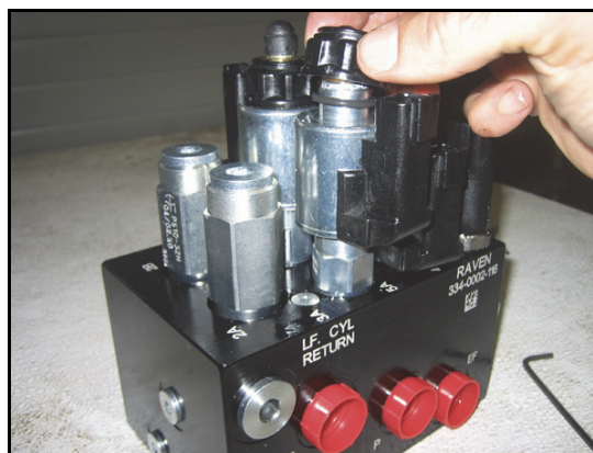
FIGURE 6. Coil Reinstalled on the AutoBoom Valve
