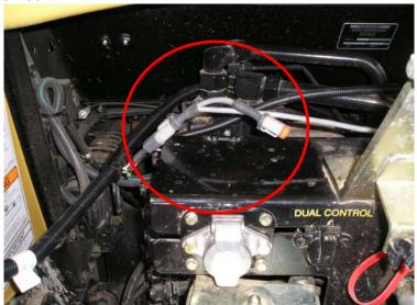
d. Connect a CAN Terminator P/N 063-0172-369 to the remaining open CAN connector.
