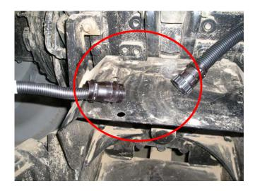
b. Connect CAN AccuBoom/Serial Console Cable P/N 115-1001-004 between the two connectors previously disconnected.
