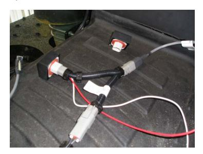
c. Connect one of the connectors on the other end of the CAN Tee Cable to the CAN connector on the CAN AccuBoom Cable P/N 115-1001-004.
