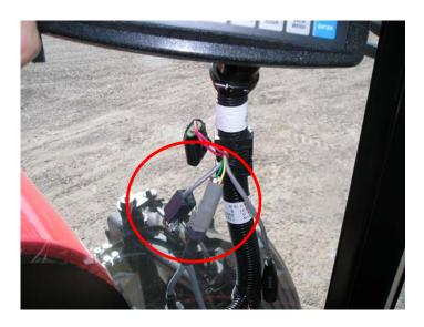
d. Connect a CAN Terminator P/N 063-0172-369 to the remaining open CAN connector near the console.
