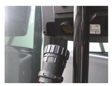
b. Connect CAN AccuBoom/Serial Console Cable (P/N 115-1001-005) to the back of the SCS4400 console.
