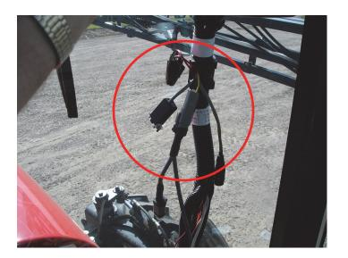
d. Connect a CAN Terminator (P/N 063-0172-369) to the remaining open CAN connector near the SCS4400 console.
