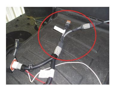
c. Connect the CAN connector on the AccuBoom cable (P/N 115-1001-005) to the remaining open CAN connection on the selected CAN Tee Cable.
