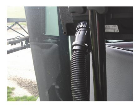
c. Connect the console cable previously disconnected to the mating connector on CAN AccuBoom/Serial Console Cable (P/N 115-1001-005).
