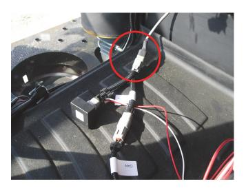
b. Break the CAN connection and insert the selected CAN Tee cable.
