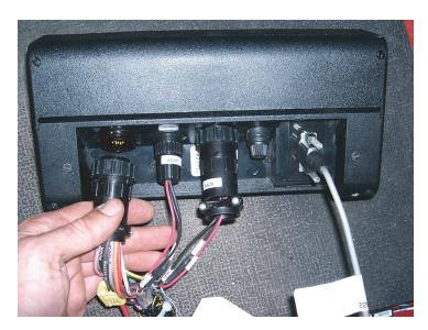
b. Connect the CAN AccuBoom/Serial Console Cable P/N 115-1001-003 to the back of the Raven console.
