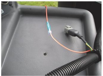
c. Connect the other end of the wire to the output of the master spread/hold switch.
