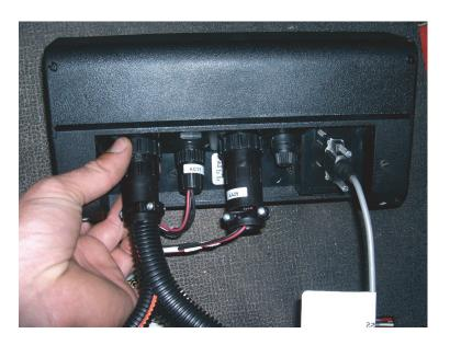
c. Connect the console cable previously disconnected to the mating connector on the CAN AccuBoom/Serial Console Cable P/N 115-1001-003.
