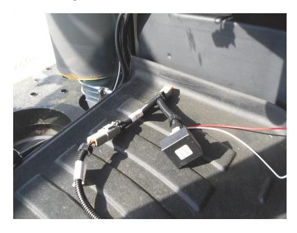
The CAN bus system is now installed and CAN nodes may be connected to it.
