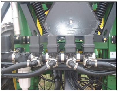
b. Distributed Valves - If the boom valves are located along the length of the boom, you will need to make extension cables to connect from the CAN AccuBoom Universal cable (P/N 115-0171-488) to the individual boom valves
