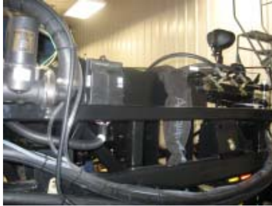
Mount Accuboom Node to center rack.
