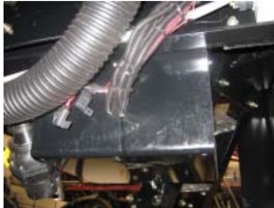
Connect larger pwr/gnd wires to battery.
