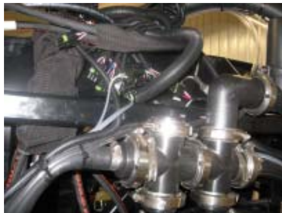
Connect Accuboom harness to boom valves
