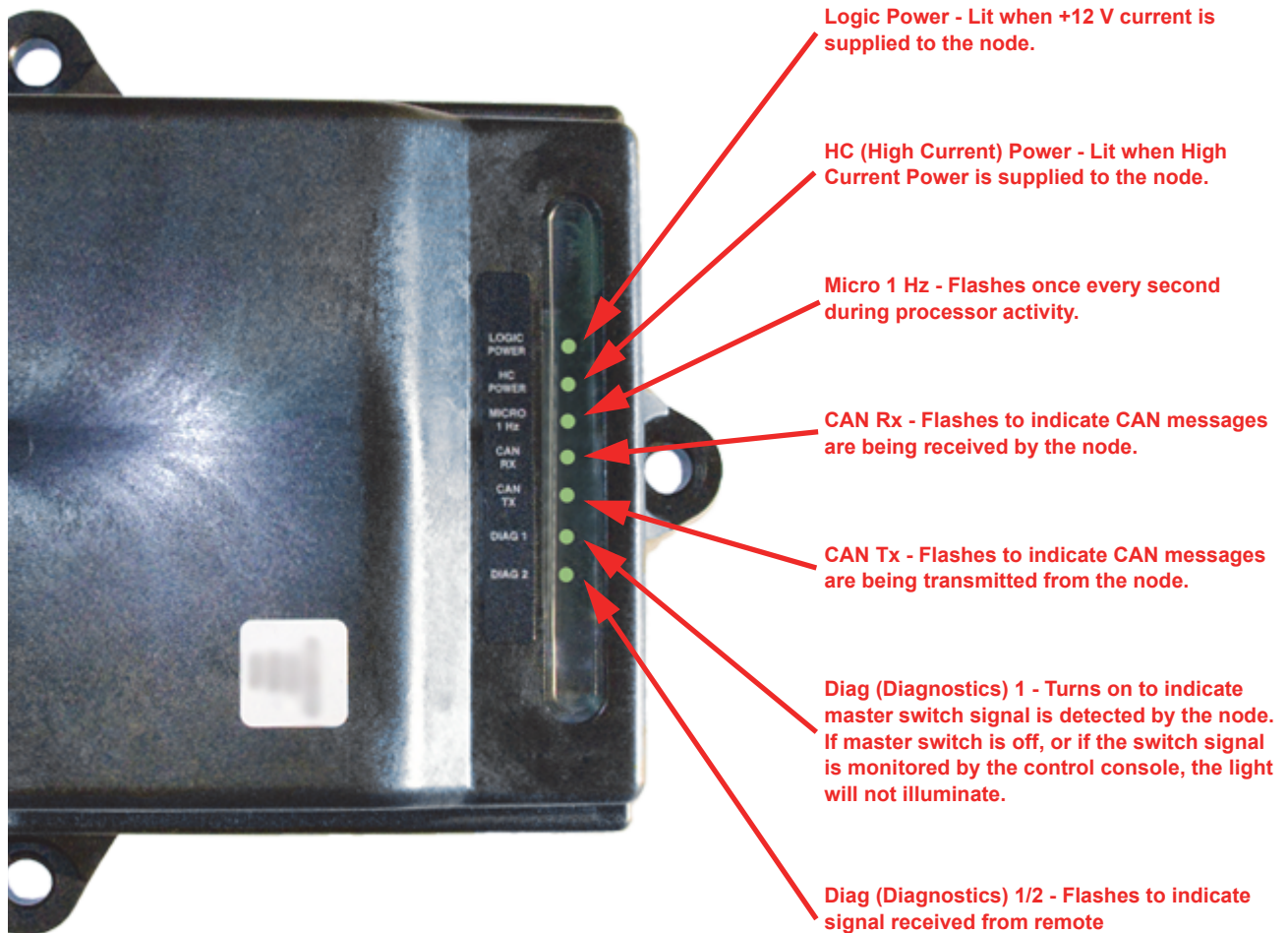
FIGURE 1. AccuBoom CAN Control Node LEDs
