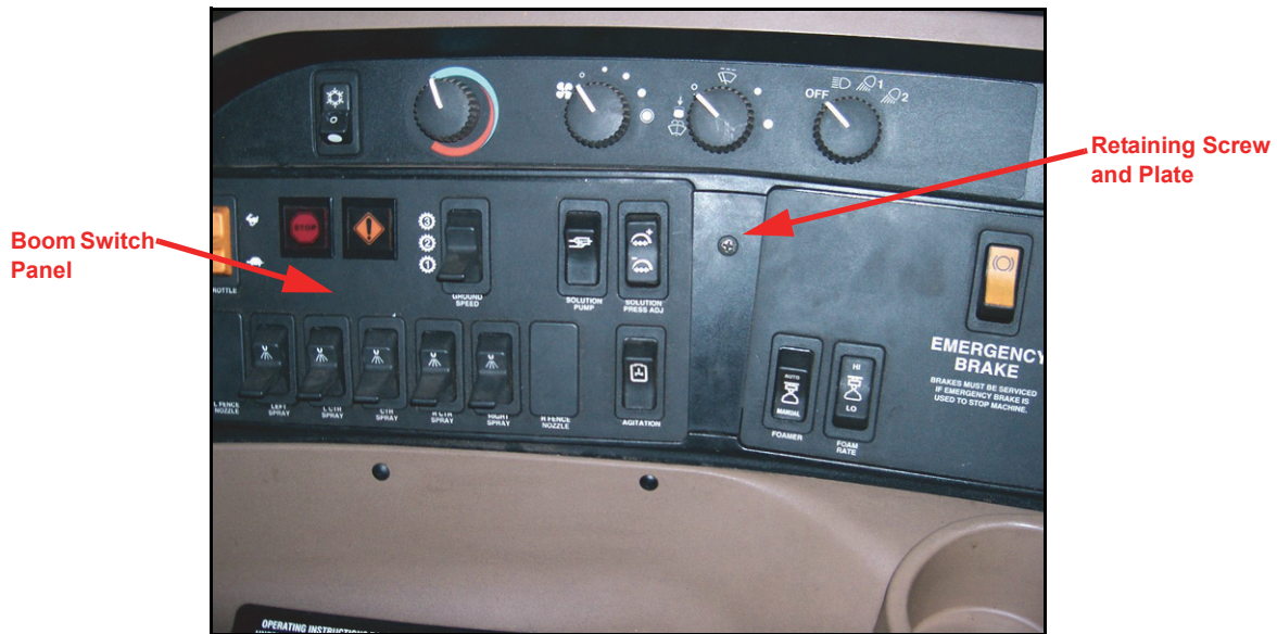
FIGURE 2. Switch Panel Access
