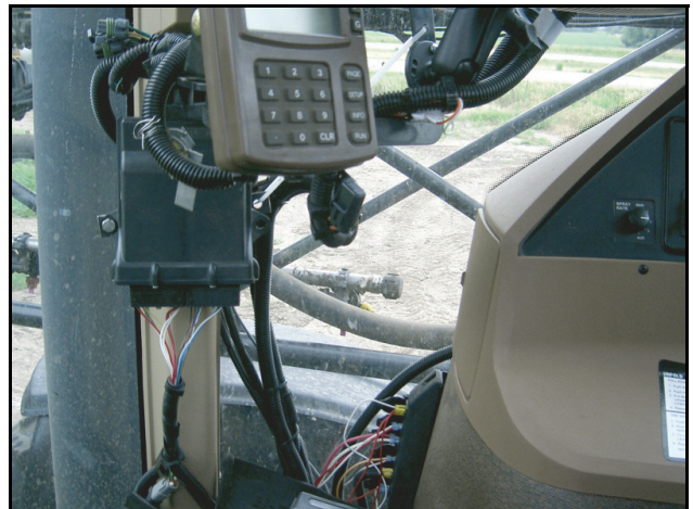
FIGURE 1. Potential AccuBoom Node Mounting Location Examples
