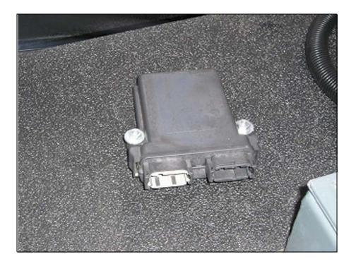
5. Connect the corresponding gray and black connectors from the Parallel AccuBoom cable (P/N 115-0171-630) to the Parallel AccuBoom node (P/N 063-0172-517).
