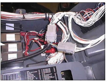
3. Connect the Parallel AccuBoom Cable (P/N 115-0171-630) to the Viper communication port.
