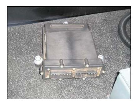
3. Connect the CAN AccuBoom cable (P/N 115-0171-631) to the CAN AccuBoom Node (P/N 063-0172-316).
