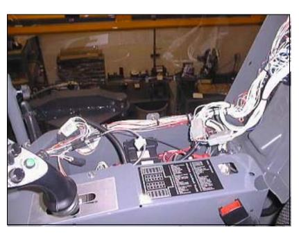
b. Locate the booms switch interface connectors. These are 12-pin rectangular Deutsche connectors.
