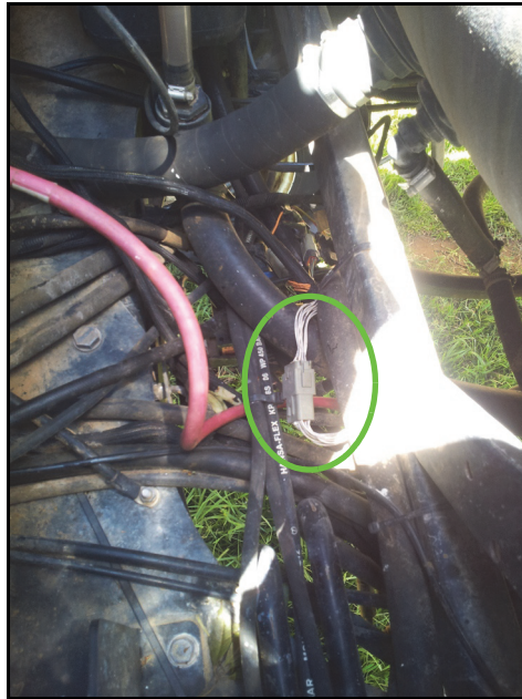
FIGURE 9. FIGURE 6. Fence Row Nozzle Connection
