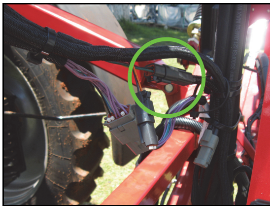
FIGURE 5. Machine's Existing CAN Connection
