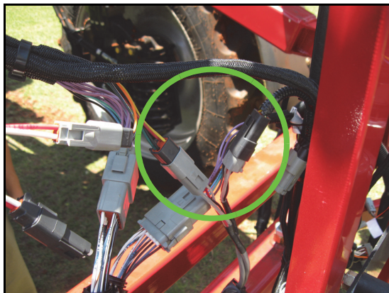
FIGURE 6. AccuBoom Harness Installed on Machine's CAN Connections
