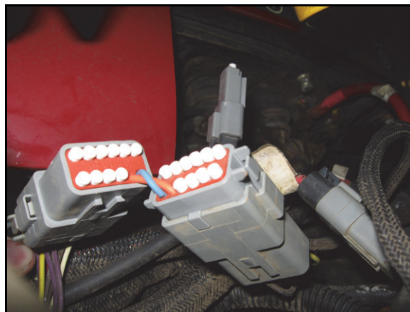
FIGURE 7. Fence Row Adapter Cable Installed
