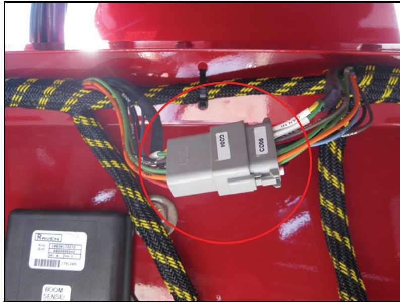
FIGURE 2. Deutsch Connectors on the Chassis Harness
