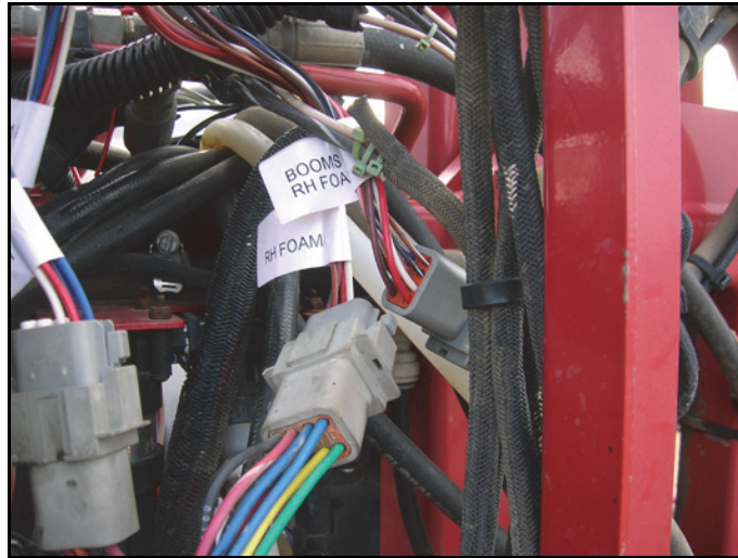
FIGURE 2. AccuBoom™ Control Cable (P/N 115-0171-667) Installed
