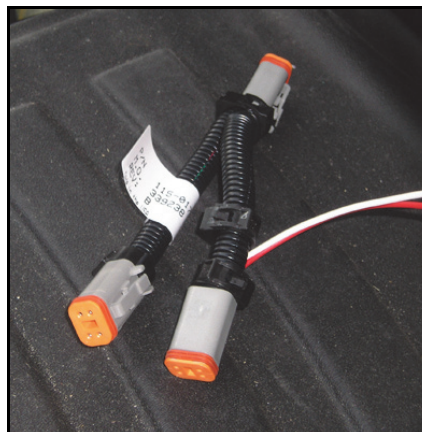
FIGURE 1. CAN Adapter Tee Cable with Power (P/N 115-0171-368)
