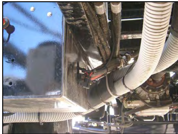
Figure 5: Connect Power Lead to the Battery.
