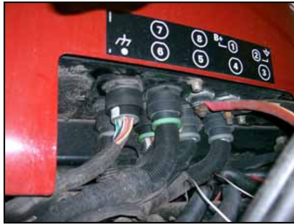
FIGURE 2. AccuBoom Harness Cable Installed
