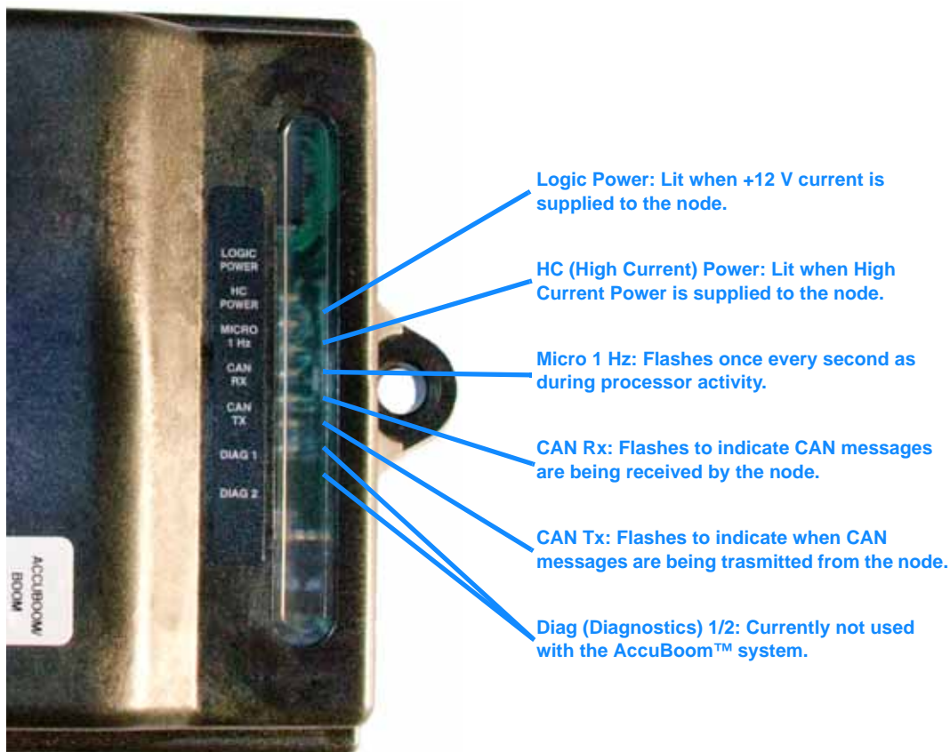
FIGURE 1. AccuBoom™ CAN Control Node (P/N 063-0172-316)
