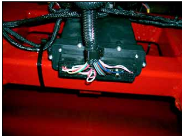
FIGURE 2. AccuBoom™ Node Connections
