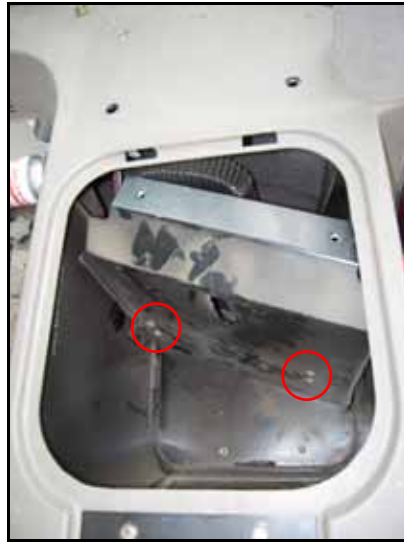
FIGURE 3. Bolts Securing the Motor to the Panel
