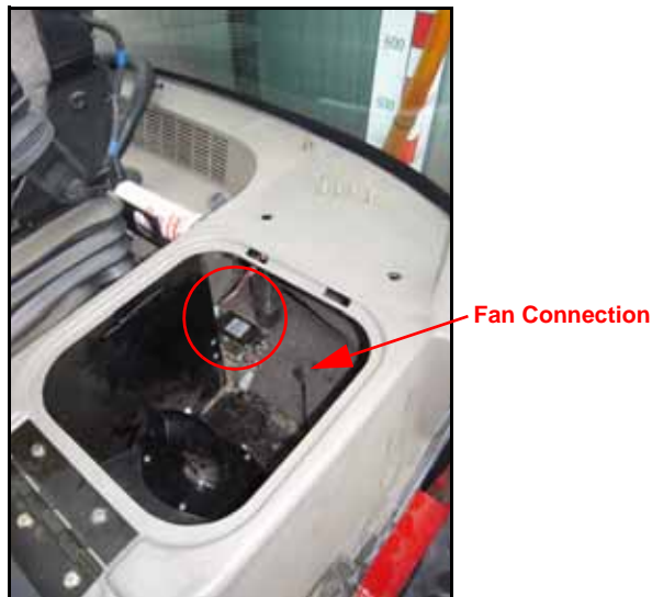
FIGURE 4. AccuBoom Filter Installation Location
