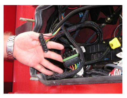
4. Plug the mating connectors from the CAN AccuBoom cable P/N 115-1001-011 to the corresponding connectors previously disconnected.
