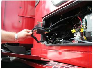
3. Disconnect the 6 pin boom connections.
