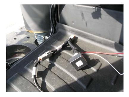
The CAN bus system is now installed and CAN nodes may be connected to it.
