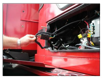
3. Disconnect the 6-pin boom connections.
