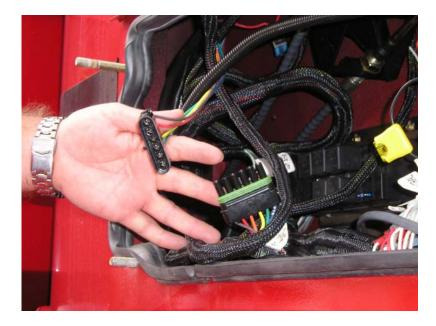
3. Disconnect the 6-pin boom connections.
