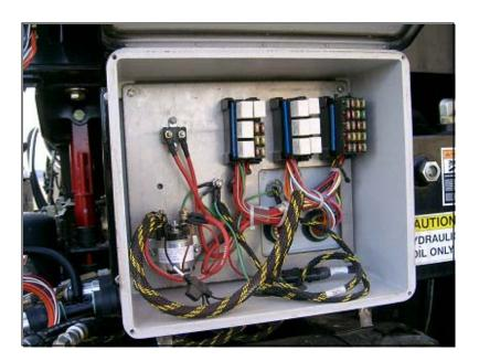
f. Drill a hole in the side of the box and route the red and white power and the ground wires through the previously drilled holes. Seal the wires and the hole using silicon caulk.
