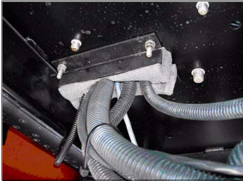
Can cable routed into cab from bottom side of cab
