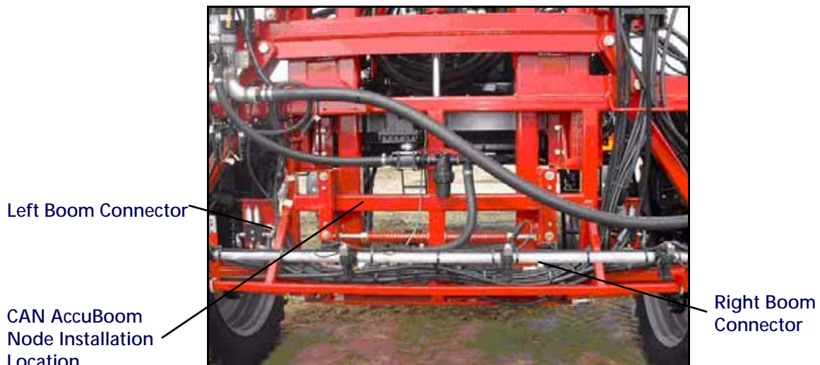
FIGURE 1. CAN AccuBoom Node Installation Location
