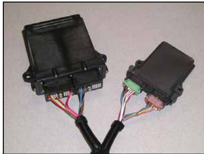
FIGURE 3. AccuBoom Cable Connected to Node and H-Driver
