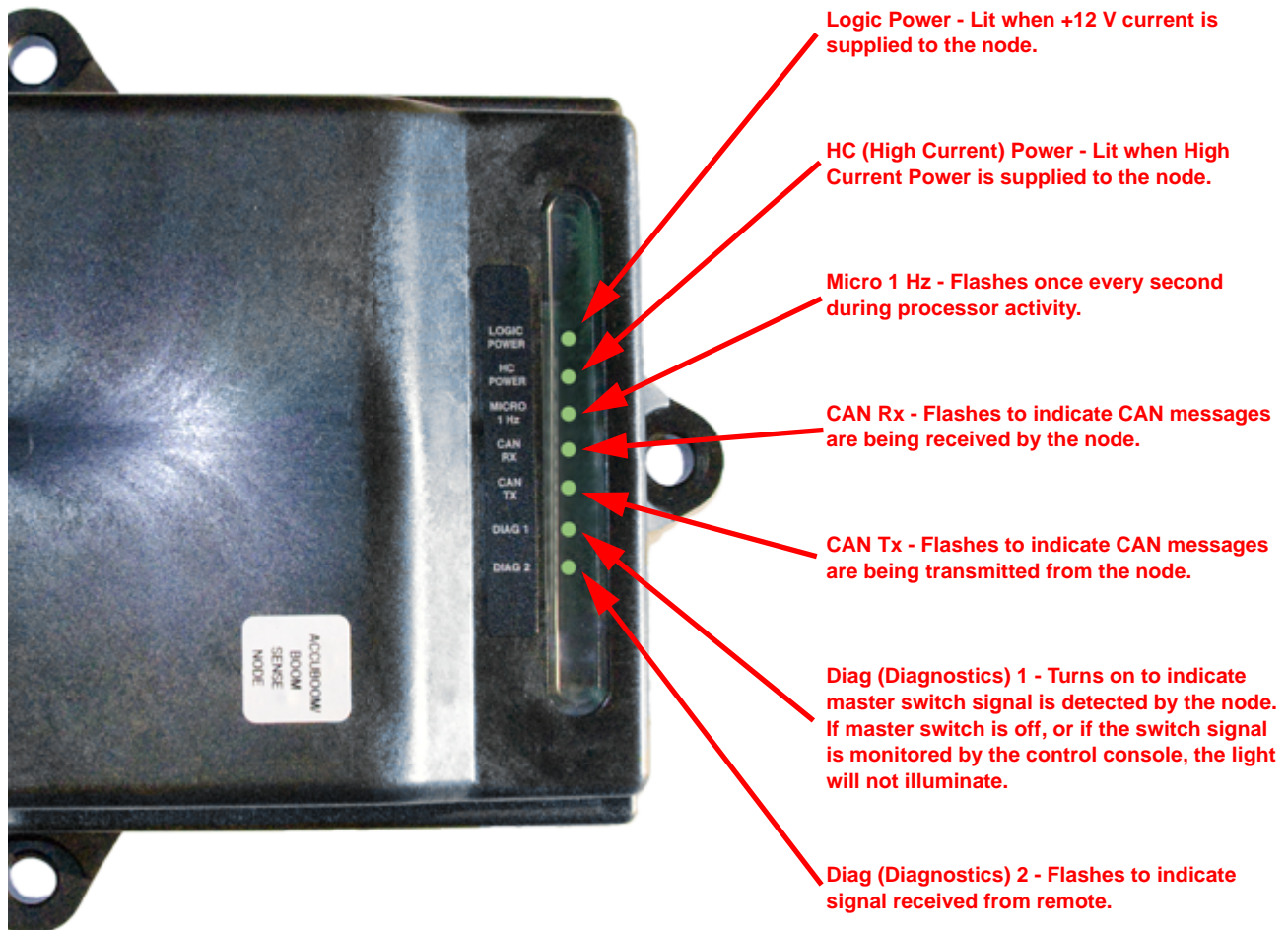
FIGURE 1. AccuBoom CAN Control Node LEDs
