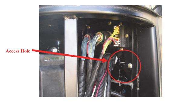
8. Remove the side access panel located on the lower left side of the operator cab.
