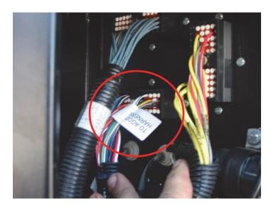
b. Tee in the AccuBoom Cable P/N 115-1001-006 between the Rogator boom cable bulkhead connector and the boom harness cable.
