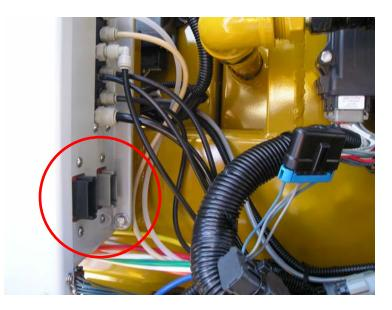
b. Tee in the AccuBoom Cable P/N 115-0171-701 between the Terragator boom cable and the boom harness cable.
