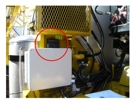
3. Connect AccuBoom cable to the sprayer boom harness.a. Unplug the Terragator boom cable from the Air Box.
