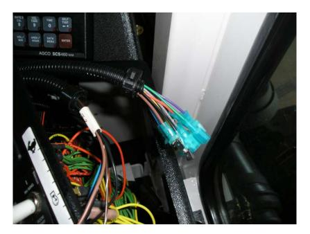
e. Remove each boom section wire from each boom switch and substitute the corresponding boom wire from the Parallel AccuBoom Cable P/N 115-0171-598 following the chart below.
